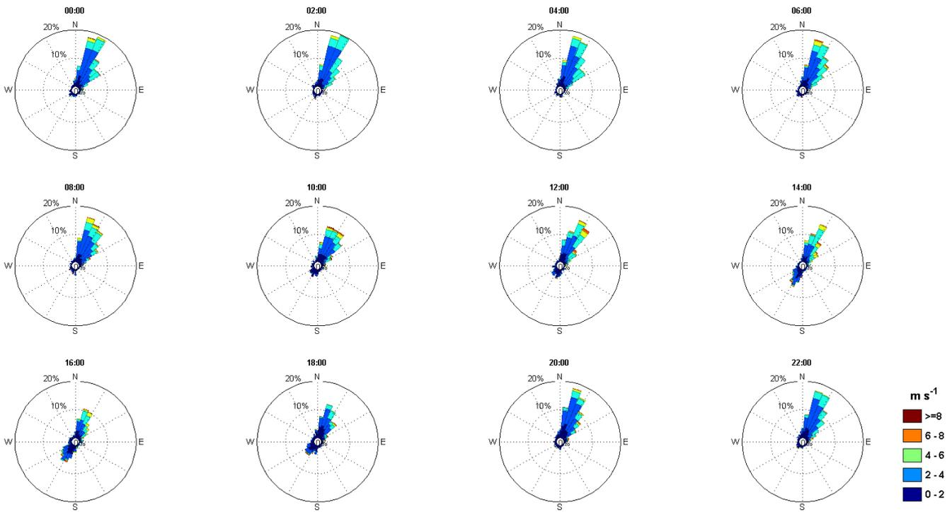
Figure 4: Hourly wind roses showing the hourly predominant wind direction and the wind speed frequency at AWS1 (local time).
