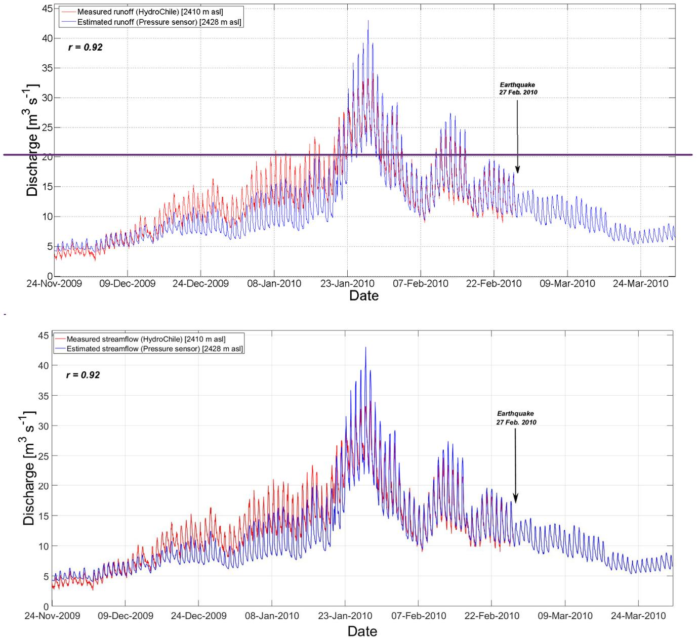
5 **Figure 10:** Time series of hourly runoff-discharge in the proglacial stream from the water level pressure sensor and the HydroChile gauging station.
