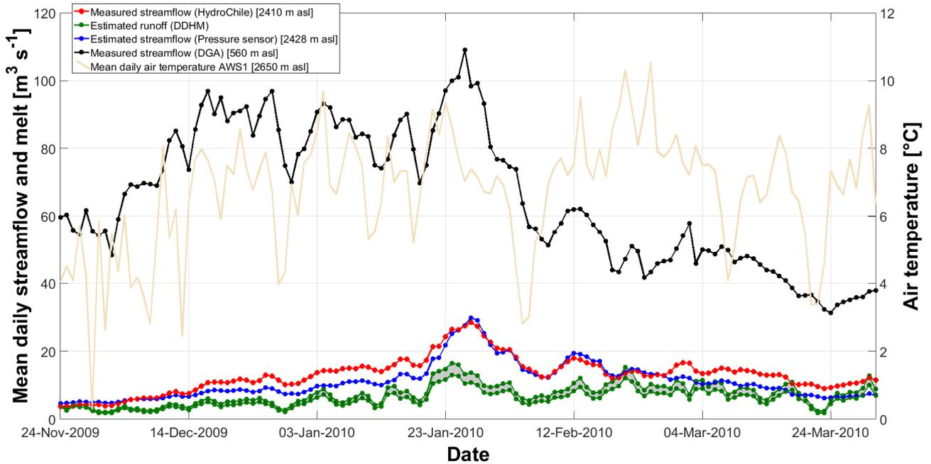
Figure 123: Daily mean runoff-melt from the distributed degree-hour model, and river runoffdischarge measurements from the water level sensor, HydroChile station and DGA station. For reference in Mean daily air temperature at AWS1 is plotted in on the right y axis.
