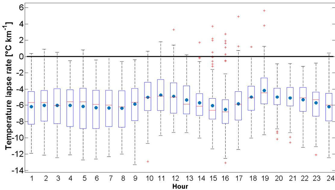
10 Figure 3: Boxplot showing the statistical distribution of hourly lapse rates calculated between AWS1 and AWS2 in the common period. Upper and lower box limits are the 75% and 25% quartiles, the red horizontal line is the median, the filled circle is the mean, and crosses are outlying values.
