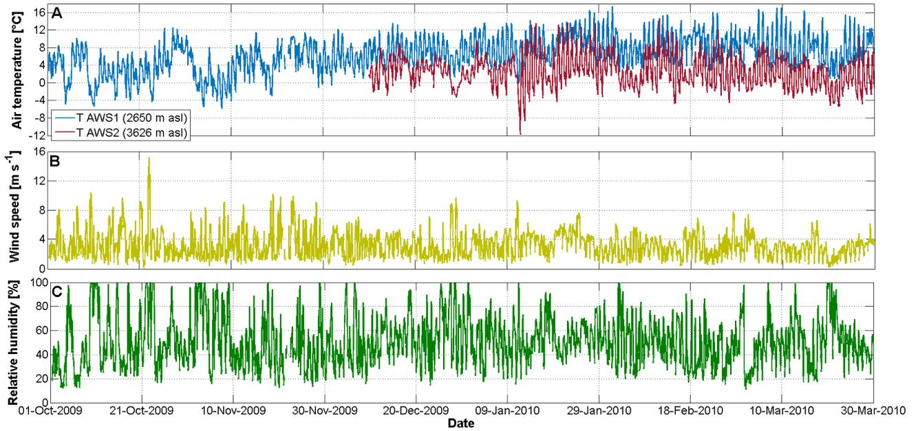
5 Figure 2: Hourly time series of hourly-observed meteorological variables observed. A) Air temperature at AWS1 and AWS2, B) Wind speed at AWS1 and C) Relative humidity at AWS1.
