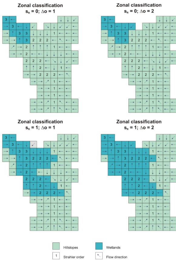
Figure A3: Sequence of parameter iteration for entire synthetic catchment. Iteration from upper left to lower right
