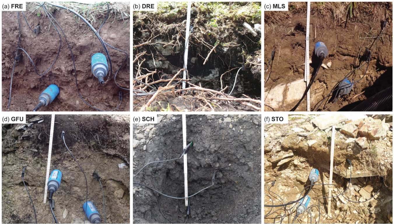
Fig. 3: Illustration of the soil characteristics and sensor installation for all SOMOMOUNT stations.
