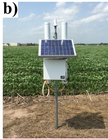
Figure 2. Eddy-Covariance Tower (a) and Cosmic-Ray Neutron Probe (b) Located at the Mead Rainfed (US-Ne3) Site.
