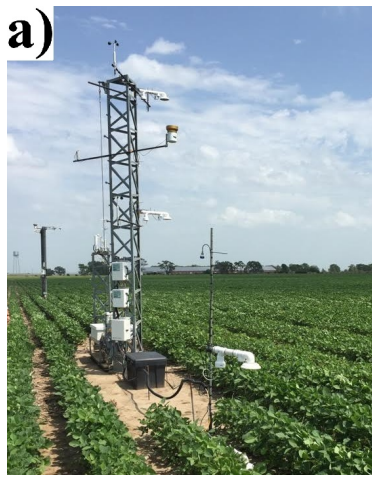
Figure 2. Eddy-Covariance Tower (a) and Cosmic-Ray Neutron Probe (b) Located at the Mead Rainfed (US-Ne3) Site.
