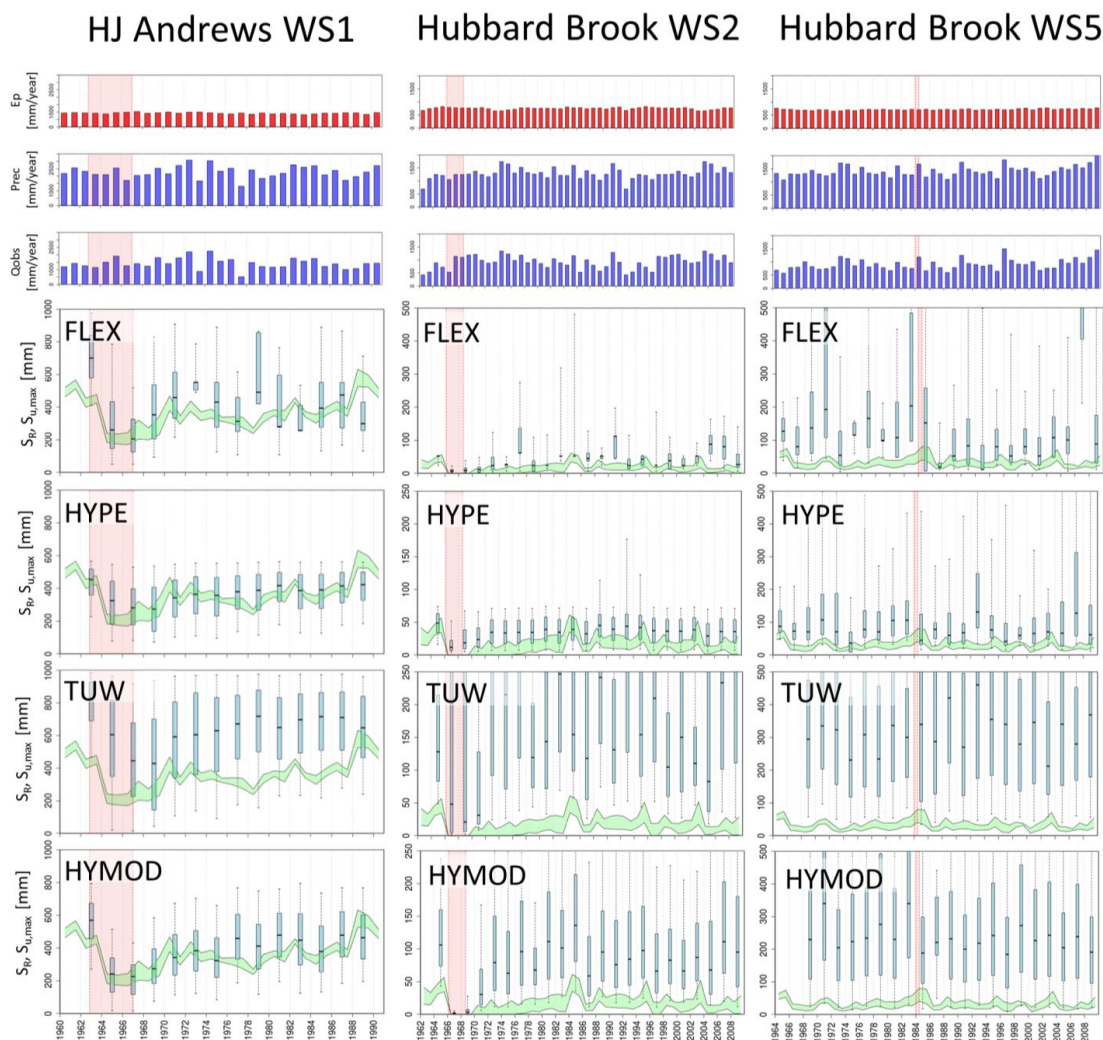
1 2 Figure 4. Evolution of root zone storage capacity S_{R,1yr} from water balance-based estimation 3 (green shaded area, a range of solutions due to the sampling of the unknown interception 4 capacity) compared with S_{u,max,2yr} estimates obtained from the calibration of four models 5 (FLEX, HYPE, TUV, HYMOD; blue boxplots) for a) HJ Andrews WS1, b) Hubbard Brook 6 WS2 and c) Hubbard Brook WS5. Red shaded areas are periods of deforestation.
