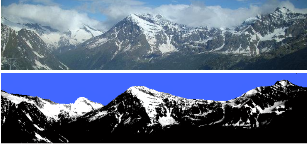
Figure 4. Example of an image (top) and the computed snow mask (bottom), where white stands for snow, black for non-snow, and blue for sky.
