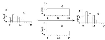
**Fig. 2.** Figure 4. Schematic of rainfall hyetograph determination in sub-basin centroid. a) Hourly hyetograph at nearest gauge, b) Daily precipitation at nearest gauge, c) Daily precipitation in sub-basin cent
