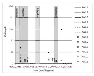
Figure 6: Modelled (solid lines) and observed (data points)  $SO_4$  concentrations without borehole leakage. High concentrations indicate admixing of deeper saltwater. Observed  $SO_4$  concentrations by far exceed the modelled concentrations.
