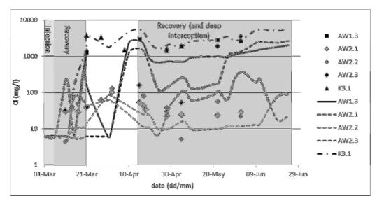
5 Figure 10: Modelled and observed Cl-concentrations at the most relevant well screens.
