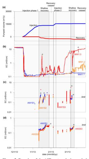
Figure 5: Pumping of the ASR system during cycle 1 (2012/2013), EC observations at MW1 (5 m from AW1), and the EC in the recovered water at AW1 and AW2. MW= monitoring well, AW= ASR well.
