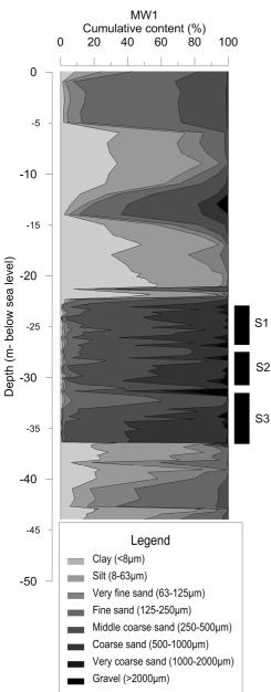
5 Figure 3: Cumulative grain size contents observed at MW1 (at 5 m from ASR well 1) in this study. S1-S3 mark the depth intervals of the ASR well screens.
