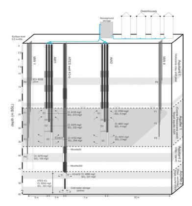
Figure 1: Cross-section of the Westland ASR site to schematize the geology, ASR wells, ATES well, and the typical hydrochemical composition of the native groundwater. Horizontal distances not to scale.
