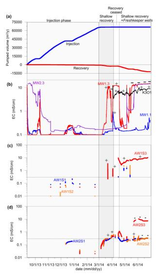
Figure 8: Pumping of the ASR system during cycle 2 (2013/2014), EC observations at MW1 (5 m from AW1), and the EC in the recovered water at AW1 and AW2. AW2.1 and AW2.3 were used for freshwater recovery (12,324 m<sup>3</sup>). Presence of increased SO<sub>4</sub>-concentrations (deep saltwater) are marked by '+', while its absence is marked by '-' (indicating shallow saltwater).
