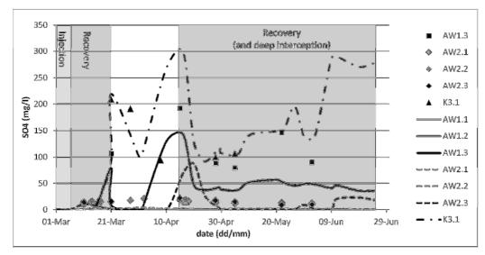
Figure 9: Modelled and observed SO<sub>4</sub>-concentrations at the most relevant well screens.
