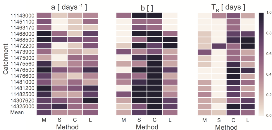
Figure 6. Results of Mann-Whitney U test sensitivity analysis. Each row represents one of the 16 study catchments, each subplot one of the three recession measures a , b , or T_R , and each subplot column one of the four methodological choices (MSCL). Each cell is colored by the fraction of statistically different pairs of shared versus unshared distributions for the particular recession measure conditioned by the two values of the corresponding method choice. A cell shading of 1 (dark purple) means all eight pairs of shared and unshared distributions were determined to be statistically different, indicating that the particular recession measure is highly sensitive to the corresponding method choice.
