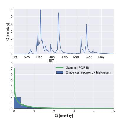
Even without including the dry season period (May – Oct) in the above PDF, the best fit gamma distribution is clearly monotonic, indicating an erratic streamflow regime.
