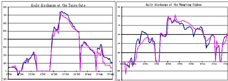
**Figure 3: Comparison between observed (solid line) and simulated (dash line) daily discharges at the Taipu Gate and Wangting Siphon (from Ou & Wu, 2001)**
