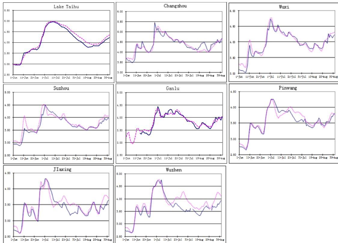
Figure 2: Comparison between observed (solid line) and simulated (dash line) water levels at eight representative stations (from
