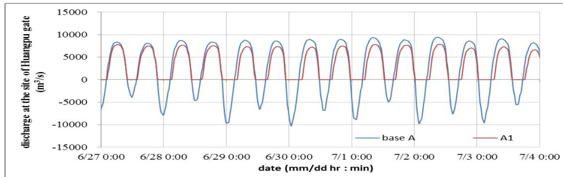
**Figure 7: Comparison of discharges at the site of the proposed gate between the scenarios base A and A1 from June 27th to July 3rd (negative discharges means the tidal water intrusion)**
