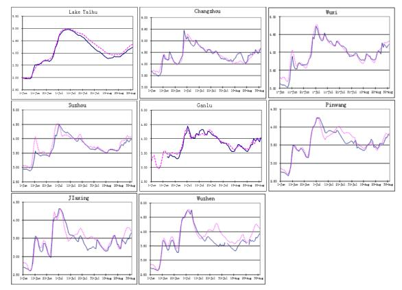
Figure 2: Comparison between observed (solid line) and simulated (dash line) water levels at eight representative stations (from 5 Ou & Wu, 2001)
