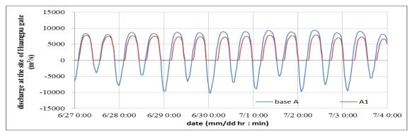
Figure 7: Comparison of discharges at the site of the proposed gate between the scenarios base A and A1 from June 27th to July 3rd (negative discharges means the tidal water intrusion)
