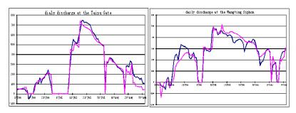
Figure 3: Comparison between observed (solid line) and simulated (dash line) daily discharges at the Taipu Gate and Wangting Siphon (from Ou & Wu, 2001)
