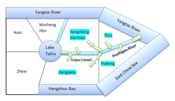
Figure 7: Conceptual drainage system along Lake Taihu – the Taipu Canal – the Huangpu River – the Yangtze River Estuary
