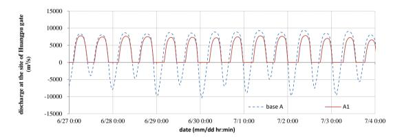
Figure 11: Comparison of discharges at the site of the proposed gate between the scenarios base A and A1 from June 27th to July  $3^{rd}$ , 1999 (negative discharges means the tidal water intrusion)
