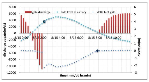
5 Figure6: A test example when the gate needs to be closed due to the high water higher than tide threshold in this tidal period (t.l.: tide level; w.l. water level; a negative discharge indicates the tidal water intrusions)
