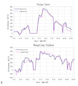
Figure 4: Comparison between daily discharges for the 1999 flood event at the Taipu Gate and Wangting Siphon (from Ou& Wu, 2001)
