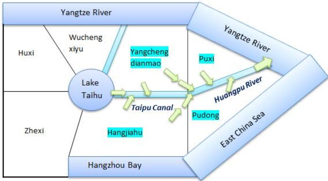
Figure 7: Conceptual drainage system along Lake Taihu – the Taiapu Canal – the Huangpu River – the Yangtze River Estuary
