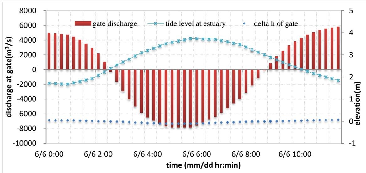
Figure5: A test example when the gate keeps open due to the high water lower than tide threshold in this tidal period (t.l.: tide level; w.l. water level; a negative discharge indicates the tidal water intrusions)
