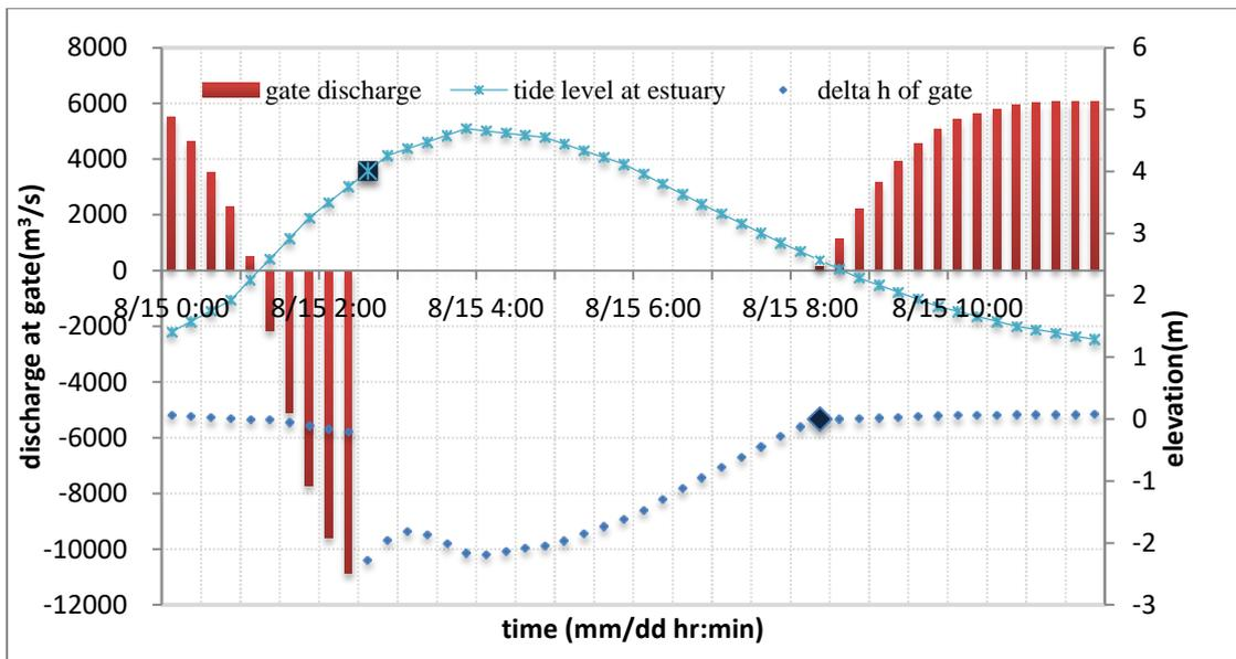
5 Figure6: A test example when the gate needs to be closed due to the high water higher than tide threshold in this tidal period (t.l.: tide level; w.l. water level; a negative discharge indicates the tidal water intrusions)
