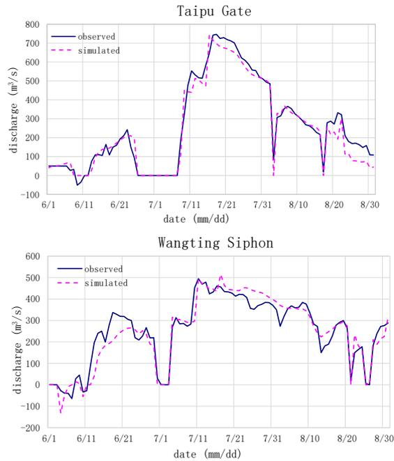
**Figure 4: Comparison between daily discharges for the 1999 flood event at the Taipu Gate and Wangting Siphon (from Ou & Wu, 2001)**
