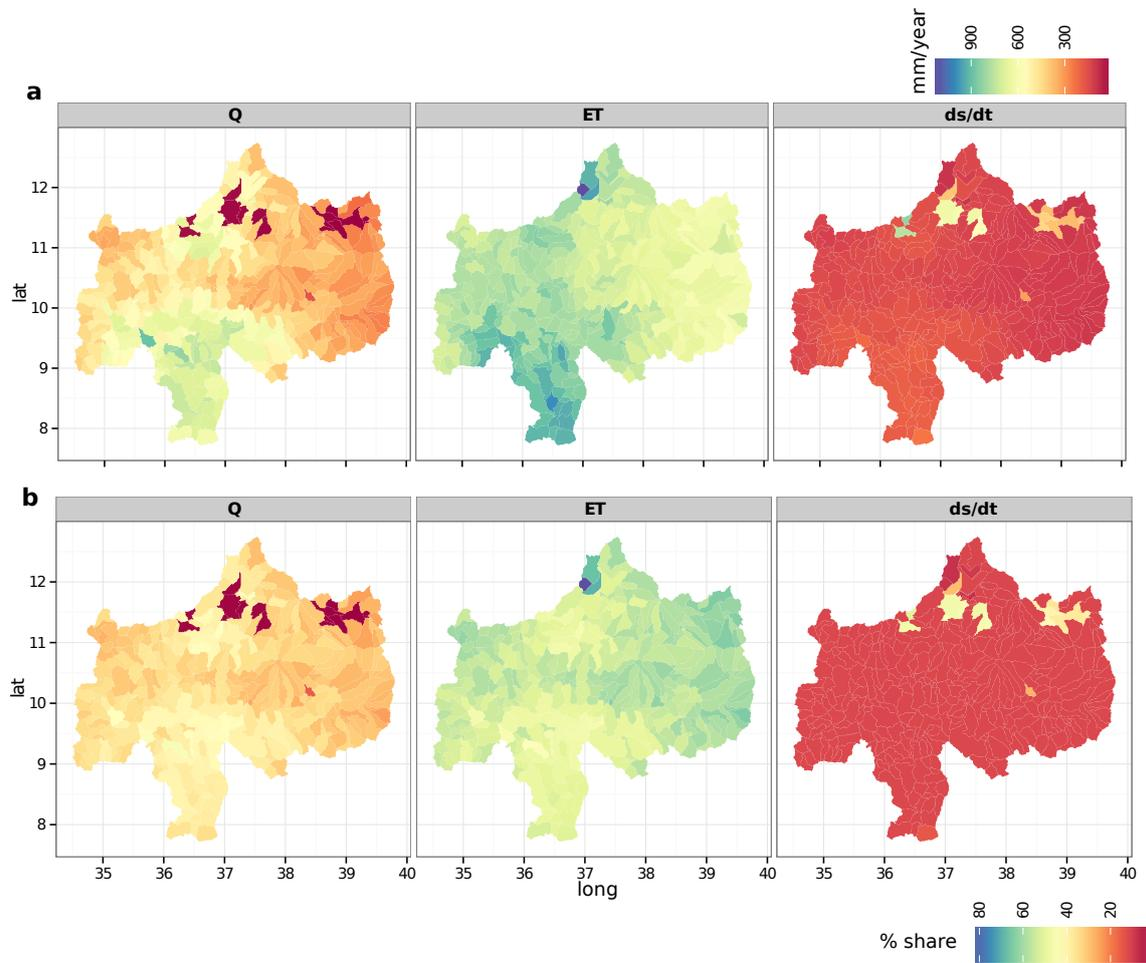
**Figure 8.** The spatial distributions of long term mean annual water budget closure: precipitation in mm (figure 3), the output terms (Q, ET,  $ds/dt$ ) in mm (a), and the percentage share of the output term (Q, ET,  $ds/dt$ ) of the total precipitation (b).
