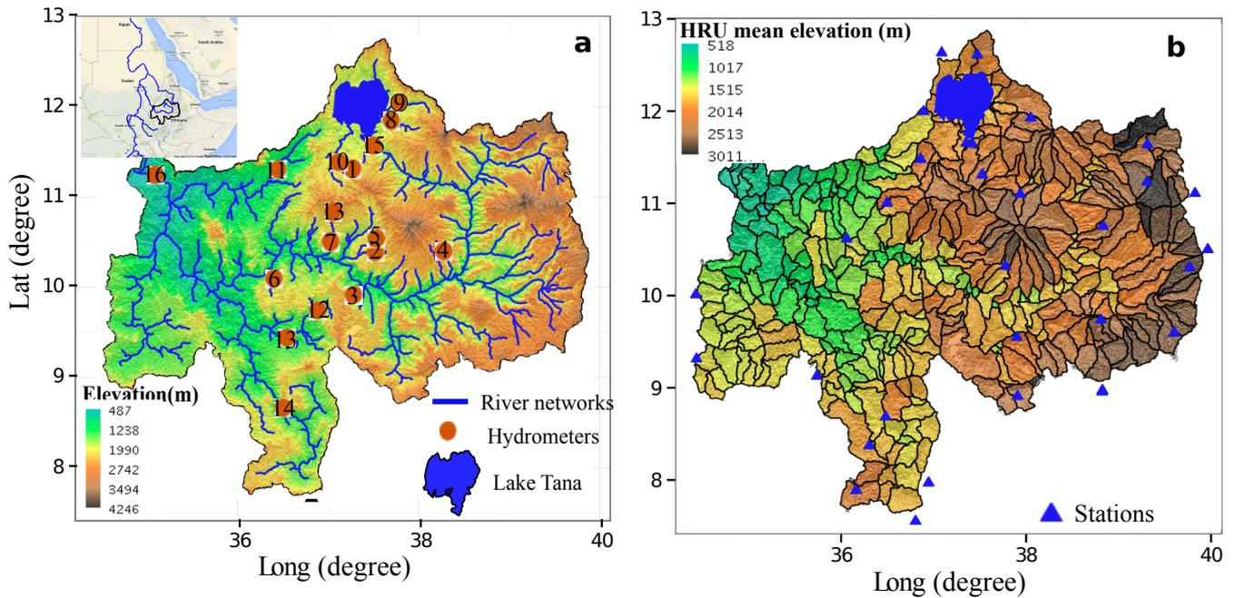
**Figure 1.** The Upper Blue Nile basin digital elevation map, along with the gauge stations (a); and subbasin partitions and meteorological stations used for simulation (b). Numbers inside the circles (figure a) designates the river gauging stations. The name of the basin referring to the numbers are provided in table 4.
