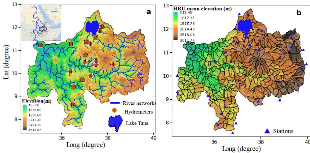
**Figure 1.** The Upper Blue Nile basin digital elevation map, along with the gauge stations (a); and subbasin partitions and meteorological stations used for simulation (b). Numbers inside the circles (figure a) designates the river gauging stations. The name of the basin referring to the numbers are provided in table 3.
