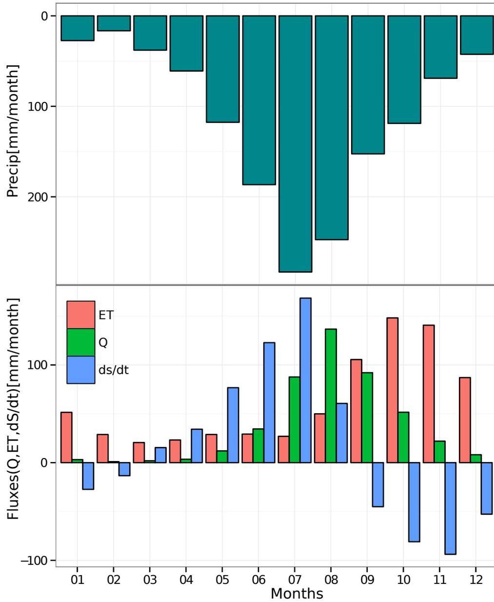
**Figure 10.** Monthly mean Water budget components at basin scale and long term, based on estimates from 1994 to 2009. The relative shares of the three components (Q, ET and dS/dt) of the total available water J are shown .
