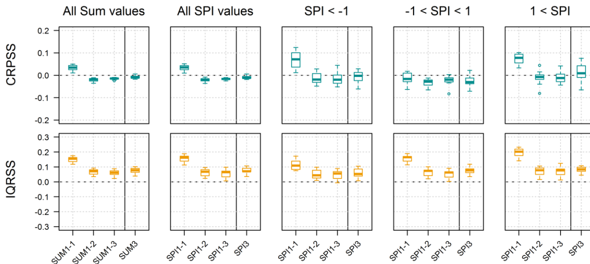
Figure 2 CRPSS and IQRSS of SPI forecasts and forecasts of cumulative precipitations produced from bias corrected System 4 precipitation forecasts. The reference for the skill scores is climatology. Skill scores are presented for statistics calculated over one month and three months altogether (Sum1 and Sum3; SPI1 and SPI3). Columns correspond to scores computed for sums, SPI values, SPI values smaller than -1 (dry), SPI values within -1 and 1 (normal) and SPI values greater than 1 (wet).
