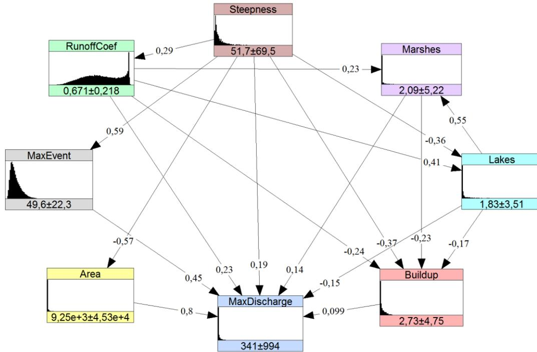
**Figure 3.** Bayesian Network for river discharges in Europe. The nodes are presented as histograms, with numbers indicating the means and standard deviations of the variables. Values on the arcs are the (conditional) rank correlation coefficients.
