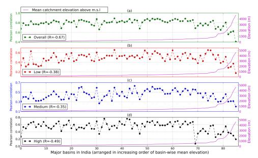
Figure 15. Graphical representation of correlation of TRMM (1998-2013) arranged in the increasing order of basin-wise average elevation over mean sea level for (a) overall time series and over (b) low, (c) medium and (d) high rainfall regime for 86 major basins in India.
