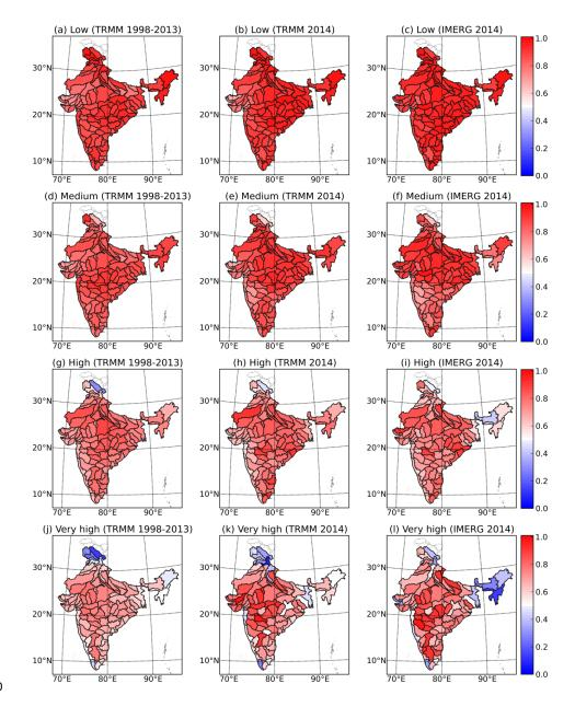
Figure 7. Spatial representation of probability of detection (POD) for (a) - (c) low (25 percentile), (d) - (f) medium (50 percentile), (g) - (i) high (75 percentile) and (j) - (l) very high (95 percentile) rainfall threshold for TRMM (1998-2013), TRMM (2014) and IMERG (2014) rainfall estimates over 86 major basins in India.
