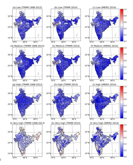
Figure 8. Spatial representation of false alarm ratio (FAR) for  $(\mathbf{a}) - (\mathbf{c})$  low (25 percentile), (d) - (f) medium (50 percentile), (g) - (i) high (75 percentile) and (j) - (l) very high (95 percentile) rainfall threshold for TRMM (1998-2013), TRMM (2014) and IMERG (2014) rainfall estimates over 86 major basins in India.
