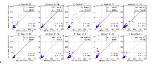
**Figure 2.2.** Scatterplot of satellite precipitation products (TRMM and IMERG) vs observed rainfall (IMD) for (**a**) – (**e**) five best basins in terms of correlation of IMERG with IMD (arranged in descending order) and (**f**) – (**j**) five worse basins in terms of correlation of IMERG with IMD (arranged in ascending order) (from March 12, 2014 to December 31, 2014).
