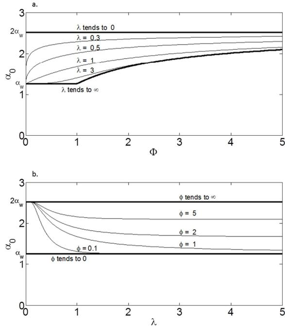
Figure 5: Variation of the Priestley-Taylor coefficient  $\alpha_0$  (Eq. (22) with  $b=1$  and  $\alpha_w = 1.26$ ): (a) as a function of the aridity index  $\Phi$  for different values of the shape parameter  $\lambda$  of the Turc-Mezentsev function; (b) as a function of  $\lambda$  for different values of the aridity index  $\Phi$ . The bold lines indicate the upper and lower limits of the feasible domain.
