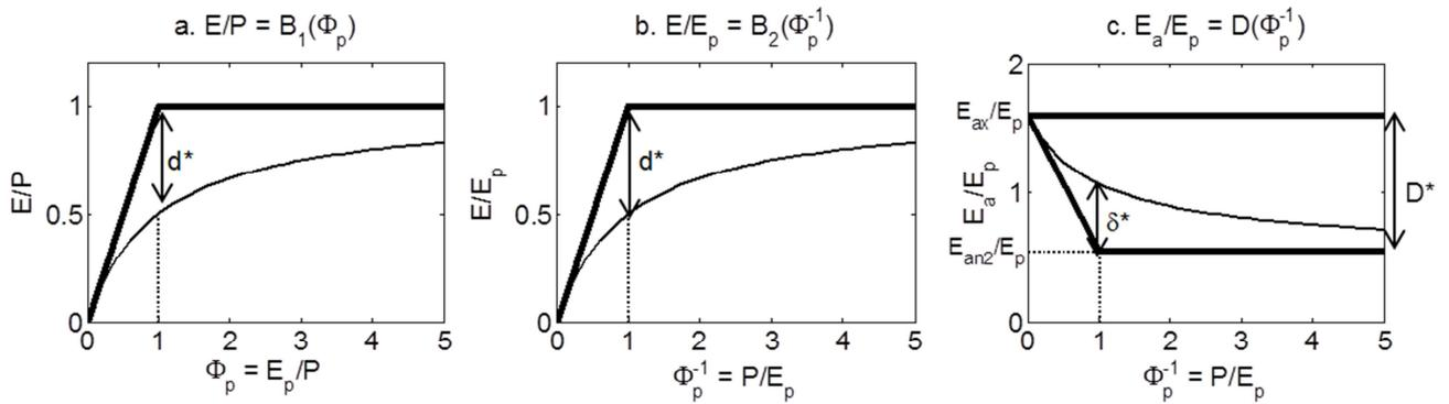
10 Figure 2: Correspondence between the two forms of the Turc-Mezentsev functions ( $E/P = B_1(\Phi_p)$  and  $E/E_p = B_2(\Phi_p^{-1})$ ) given by Eqs. (4) and (5) and the function defining the drying power of the air ( $E_a/E_p = D(\Phi_p^{-1})$ ) given by Eq. (10)). The calculations are made with  $b = 1$ ,  $\lambda = 1$  and a temperature of  $15^\circ\text{C}$ :  $d^* = 0.50$ ,  $D^* = 1.05$  and  $\delta^* = 0.52$ . The bold lines indicate the upper limit of the feasible domain.
