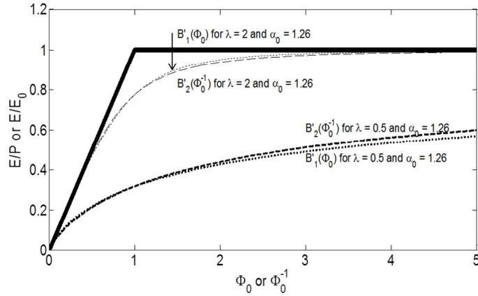
10 Figure 4: Comparison of functions  $E/P = B_I'(\Phi_0)$  (Eq. 20) and  $E/E_0 = B_2'(\Phi_0^{-1})$  (Eq. 21) for two different values of the shape parameter  $\lambda$  (0.5 and 2),  $b=1$  and  $\alpha_0 = 1.26$ .
