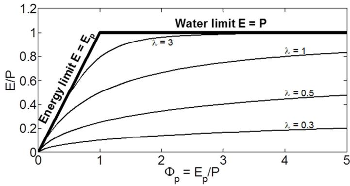
Figure 1: The Turc-Mezentsev relationship Eq. (4) between the ratio  $E/P$  and the aridity index  $\Phi_p = E_p/P$  for four values of the parameter  $\lambda$  (0.3, 0.5, 1 and 3). The bold line indicates the upper limit of the feasible domain.
