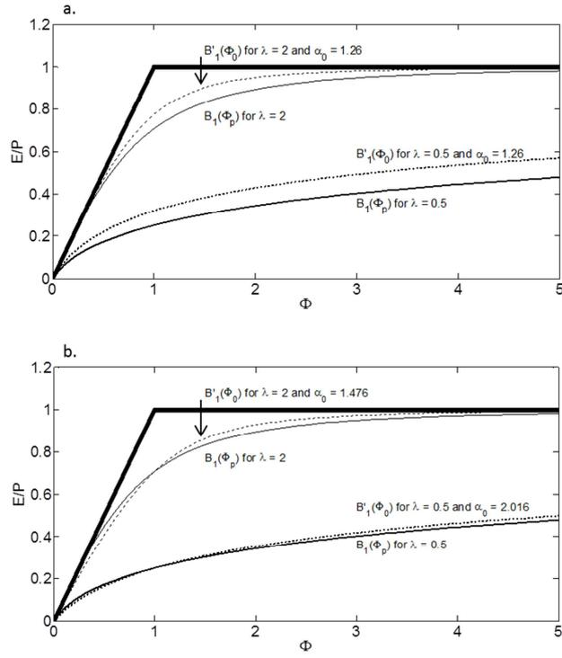
Figure 3: Comparison between the Turc-Mezentsev function  $B_I(\Phi_p)$  (Eq. 4) in solid line and its corresponding function  $B_I'(\Phi_0)$  (Eq. 20) in dotted line for two values of  $\lambda$  (0.5 and 2) and  $b=1$ : (a) with  $\alpha_0 = \alpha_w = 1.26$ ; (b) with  $\alpha_0$  adjusted according to Eq. (22) for  $\Phi = 1$ . The x-axis legend  $\Phi$  represents either  $\Phi_p$  for  $B_I(\Phi_p)$  or  $\Phi_0$  for  $B_I'(\Phi_0)$ .
