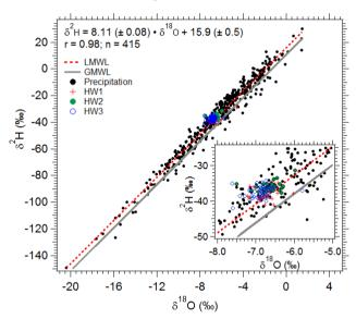
Fig. 4. Linear fit representing the LMWL for the relationship between  $\delta^2 H$  vs.  $\delta^{18}O$  in daily precipitation samples (dashed red line) and cave dripwaters (HW1, HW2, HW3). The solid grey line denotes the position of the GMWL.
