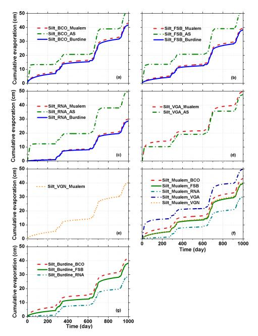
Figure 5: Cumulative evaporation from a silt soil column for the different combinations of soil water retention and hydraulic conductivity parameterizations. Panels a through e present the results for the indicated retention parameterizations (see Table 1). Panels f and g organize the results according to the conductivity function: either Mualem (1976) (f) or Burdine (1953) (g).
