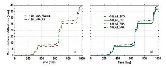
Figure 6: Cumulative infiltration in a silt profile for the VGA parameterization (see Table 1) with conductivity functions according to Mualem (1976) and Alexander and Skaggs (1986) (a) and four different parameterizations for the retention curve (see Table 1) with the Alexander and Skaggs conductivity function (b).
