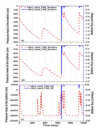
Figure 9: Pressure head hBot and flux density vBot at the bottom of the sand column for the FSB parameterization (see Table 1) and the conductivity functions of Mualem (1976) (a), Burdine (1953) (b) and Alexander and Skaggs (1986) (c).
