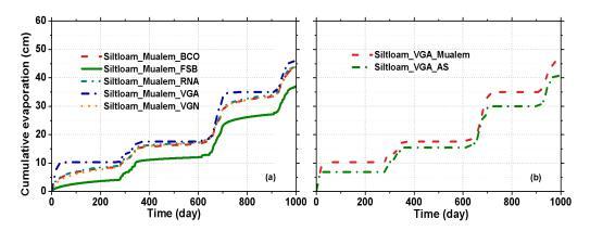
Figure 13: Cumulative evaporation from a silt loam profile for all parameterizations (see Table 1) with Mualem's (1976) conductivity function (a) and the VGA parameterization with conductivity functions according to Mualem (1976) and Alexander and Skaggs (1986) (b).
