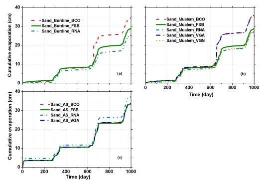
Figure 8: Cumulative evaporation from a sandy profile for the different combinations of retention curve parameterizations (see 1230 Table 1) and hydraulic conductivity functions: Burdine (1953) (a), Mualem (1976) (b) or Alexander and Skaggs (1986) (c).
