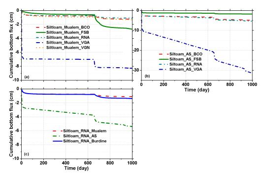
Figure 12: Cumulative bottom fluxes from a silt loam profile for all combinations of parameterizations (see Table 1) and Mualem's (1976) (a) and Alexander and Skaggs' (1986) conductivity functions (b), and for the RNA parameterization with all three conductivity functions (c).
