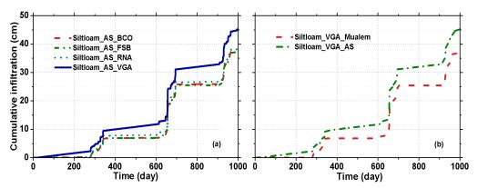
Figure 14: Cumulative infiltration from a silt loam profile for four parameterizations (see Table 1) with the Alexander and Skaggs (1986) conductivity function (a) and for the VGA parameterizations with conductivity functions according to Mualem (1976) and Alexander and Skaggs (1986) (b).
