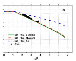
Figure 3: The observed and fitted hydraulic conductivity curve according to Burdine (1953), Mualem (1976) and Alexander and Skaggs (1986) using the fitted parameters of the Fayer and Simmons soil water retention curve (1995) for (a) sand, (b) silt, and (c) silt loam.
