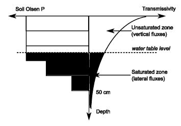
Fig. 2. Description of soil hydraulic properties and phosphorus content with depth
