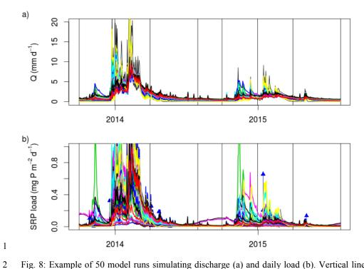
Fig. 8: Example of 50 model runs simulating discharge (a) and daily load (b). Vertical lines
