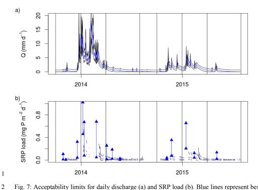
Fig. 7: Acceptability limits for daily discharge (a) and SRP load (b). Blue lines represent best estimates; black lines represent the acceptability limits. Storm loads acceptability limits are represented by vertical blue lines. Black vertical lines represent the starting and ending dates for each season (table 2).
