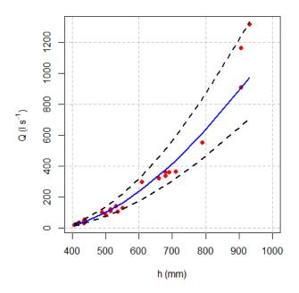
Fig. 3: Rating curve in Kervidy-Naizin; acceptability bounds derived from 90% prediction interval (blue line: fitting regression; black dots: 90% prediction interval). Red dots represent the original discharge measurements used to calibrate the stage-discharge rating curve (Carluer, 1998).
