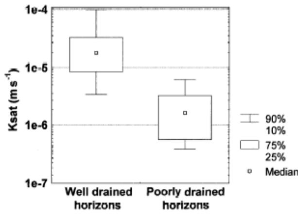
Figure 7. Saturated hydraulic conductivity of the well drained and poorly drained horizons.
