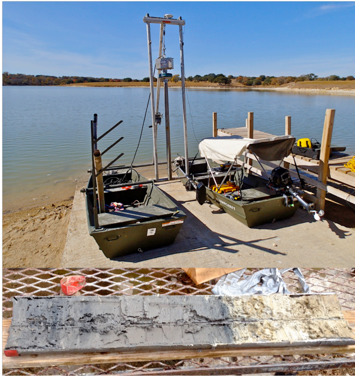
2 Figure 4. Reservoir sediment coring apparatus (top) and representative sediment profile 3 (bottom).
