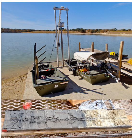
3 4 Figure 4. Reservoir sediment coring apparatus (top) and representative sediment profile 5 (bottom). 6
