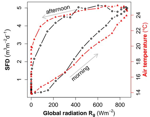
**Figure 7.** Hysteresis of sap flux density (left y-axis) and air temperature (right y-axis, red) plotted as a function of global radiation at the field site G1. Data are half-hourly values over one sunny summer day 2013-07-07. Sap flow data is taken from a beech (tree 1) at site S1.
