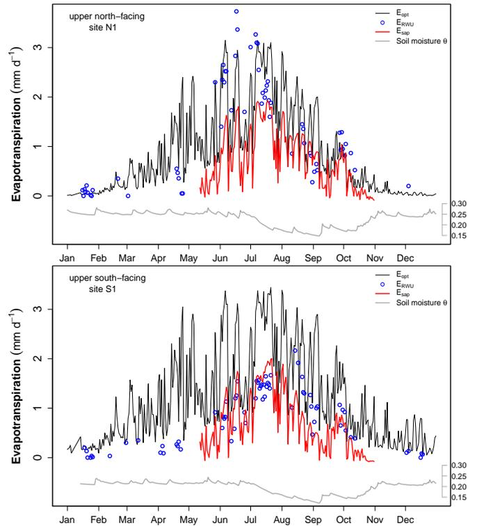
**Figure 4.** Time series of evapotranspiration estimates for north-facing hillslope site N1 in the left panel and south-facing site S1 in the right panel.  $E_{opt}$  is the potential evaporation derived from maximum power,  $E_{RWU}$  (blue points) and  $E_{sap}$  are transpiration estimates.
