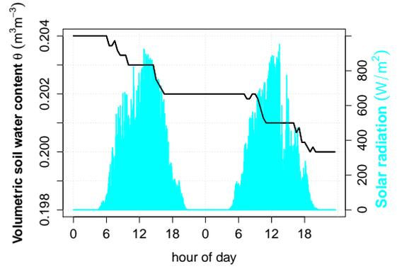
**Figure A1.** Observed diurnal decline in soil moisture over two sunny days in summer 2013 to illustrate the approach to estimate daily root water uptake from diurnal soil moisture variations.  $E_{RWU}$  is estimated at sensor level per day as a cumulative sum of differences from sunrise to sunset, in the absence of any nighttime variations or daytime increases in soil moisture.
