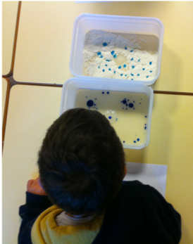
Figure 2. Design and test with artificial drops of tinted water of the flour or oil disdrometers in a classroom.
