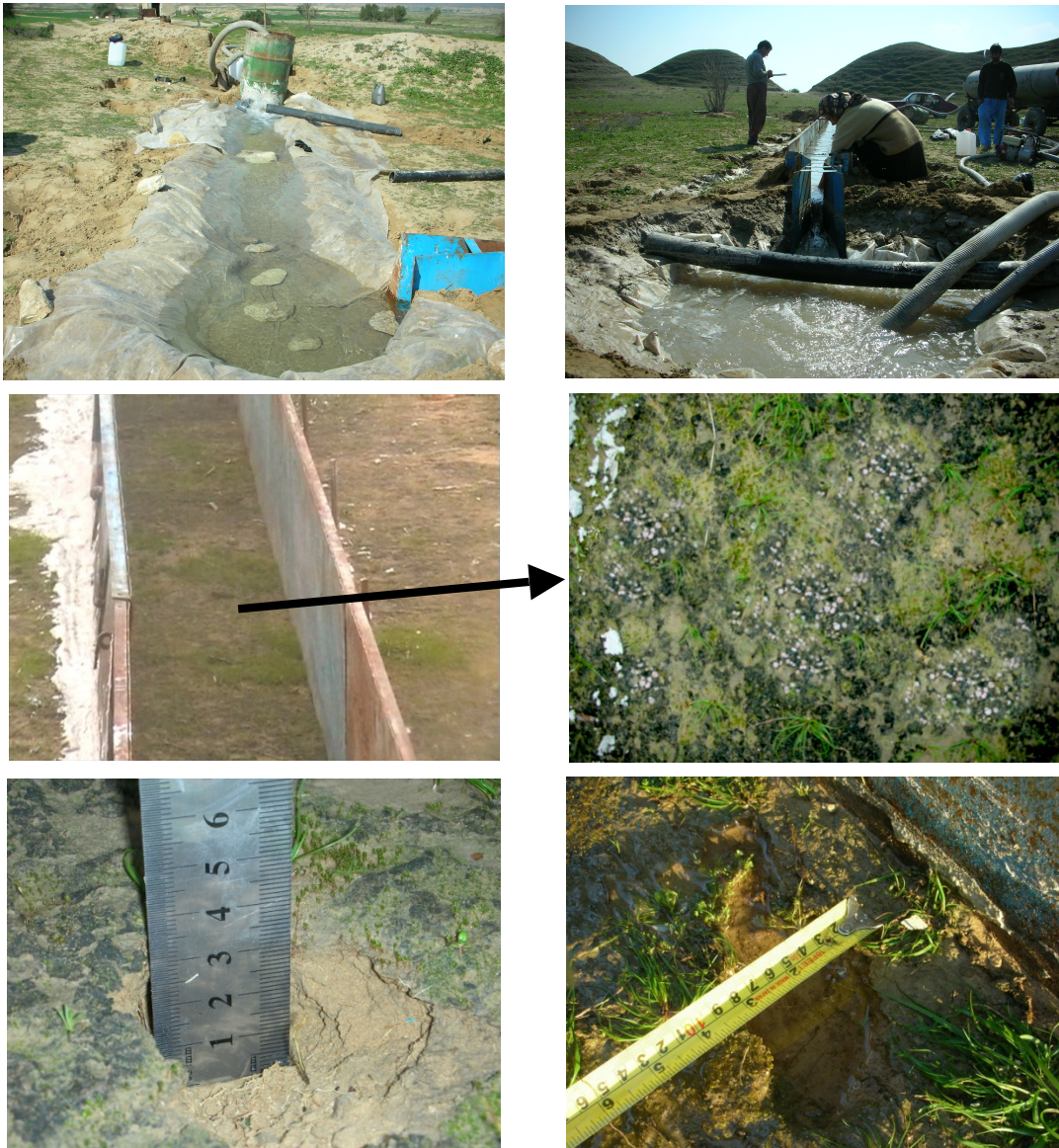
435 Fig. 1- Flume, water supply, retention pond, overflow pipe and Parshall Flume (Top 436 photos); flume surface and vegetation (grass and pale pink lichen patch) in the 437 rangeland (middle photos); sample of initiated head cut with height of 3 cm in range 438 land (bottom left) and abandoned land (bottom right).
