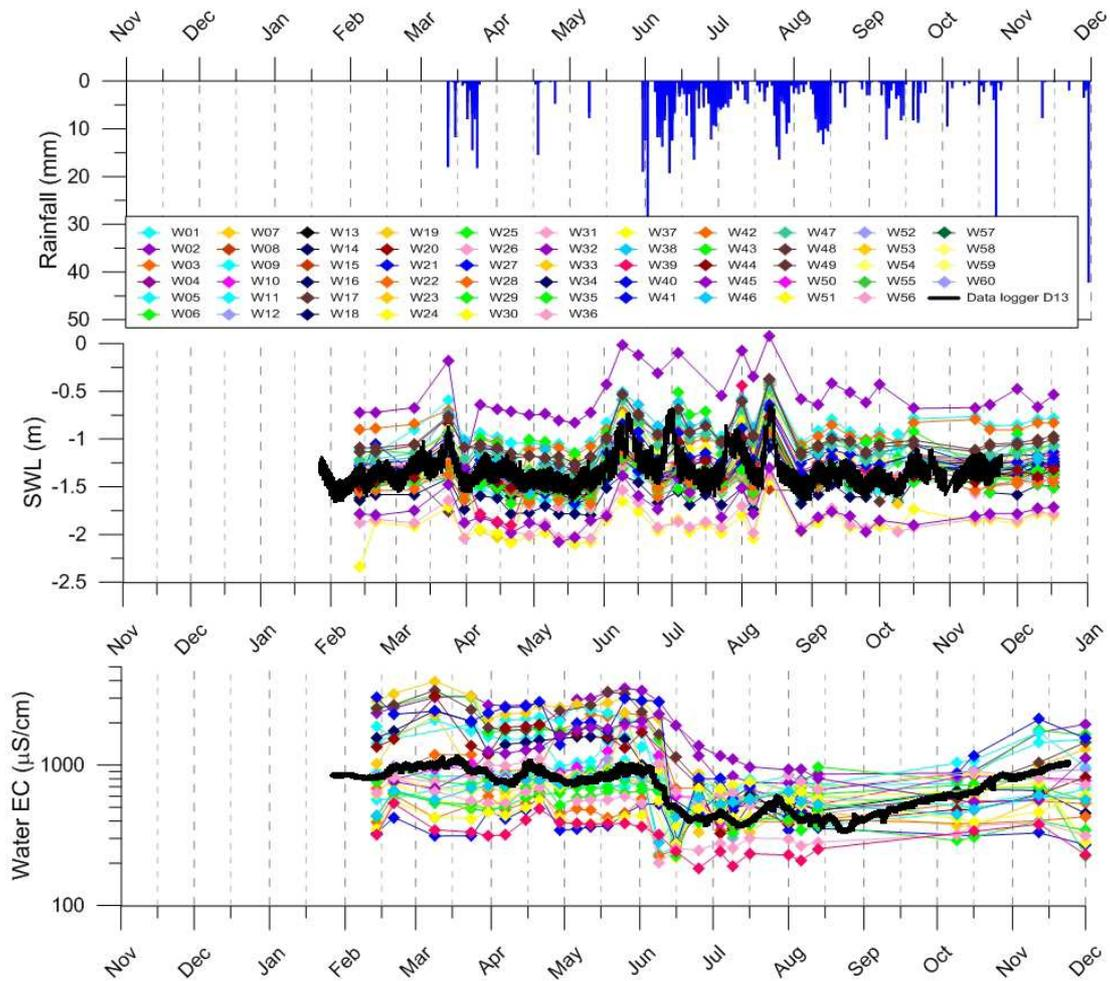
Figure 5: Rainfall, water level and EC monitoring. The black line (Data logger D13) are the data presented in the discussion paper Figure 8)
