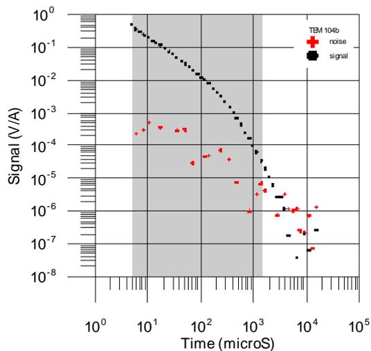
Figure 3: Example of noise and TEM measurements
