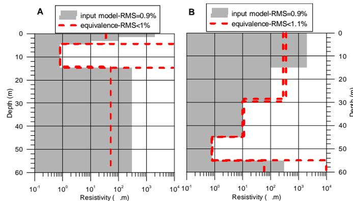
Figure 2: Equivalence and suppression of a 5 layers model. Left panel=thin layers resulting in a 3 layers output model. Right panel=thicker top layers resulting in a 4 layers output model. 1% of added noise to the synthetic data.
