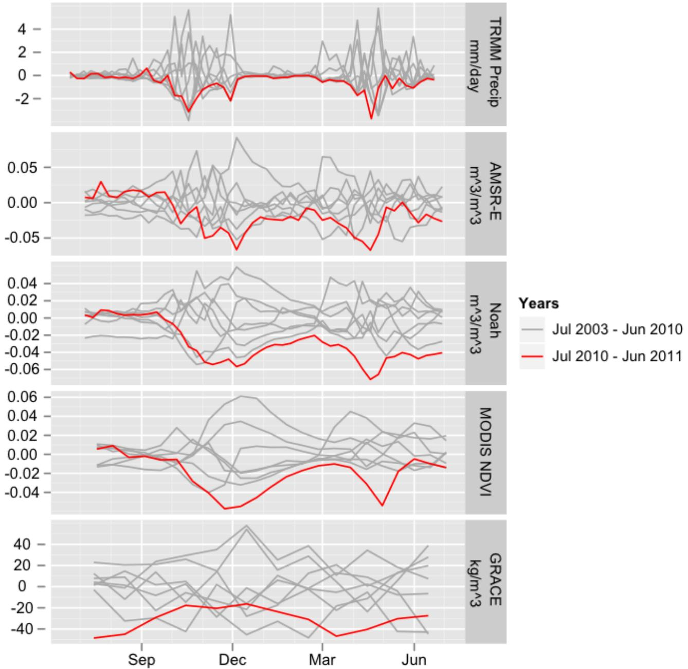
**Figure 3:** Anomaly analysis of TRMM precipitation, LPRM and Noah soil moisture estimates, MODIS NDVI and GRACE terrestrial water storage using a Jan 2003 to Jun 2010 baseline.
