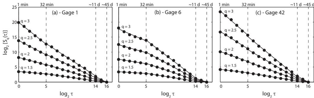
**Fig. 4.** Example of scale invariance regimes for gages with ID 1, 6 and 42 – subplots (a), (b) and (c), respectively. The slopes of the lines are estimates of the multifractal exponents  $K(q)$  in Eq. (3).
