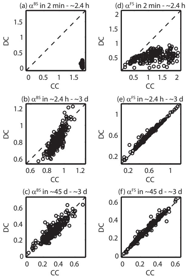
**Fig. 9.** Scatterplots between the spectral exponents computed from the signal sampled with CC (x-axis) and DC (y-axis) methods. Panels (a)–(c) (d–f) are referred to  $\alpha^{\text{BS}}$  ( $\alpha^{\text{FS}}$ ) in the three scaling regimes.
