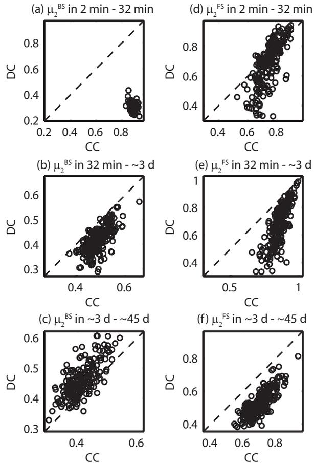
**Fig. 10.** Scatterplots between the intermittency exponents computed from the signal sampled with CC (x-axis) and DC (y-axis) methods. Panels (a)–(c) (d–f) are referred to  $\mu_2^{BS}$  ( $\mu_2^{FS}$ ) in the three scaling regimes.
