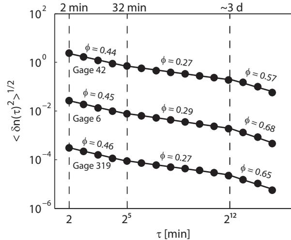
**Fig. 5.** Example of scaling regimes revealed by the computation of the clustering exponent  $\phi$  for gages with ID 42, 6, and 319. The slopes of the lines are estimates of  $\phi$  in Eq. (4). Arbitrary units in the y-axis are used in order to display results from different gages in the same graph.
