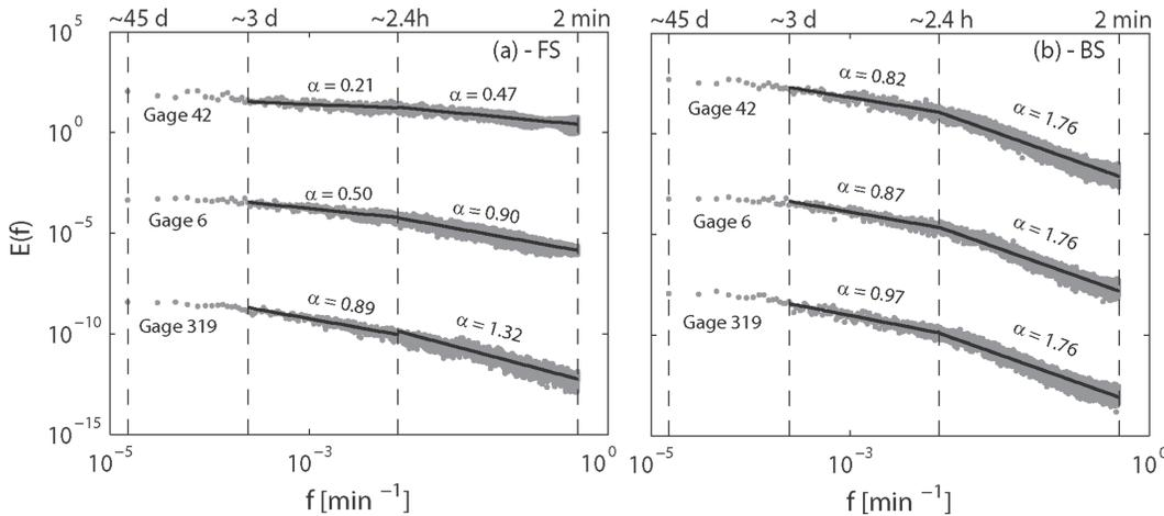
**Fig. 3.** Example of scaling regimes emerged through the spectral analysis for gauges with ID 42, 6 and 319, for **(a)** the FS and **(b)** the BS series. The slopes of the lines are estimates of the spectral exponents  $\alpha^{\text{FS}}$  and  $\alpha^{\text{BS}}$  in Eq. (1). Arbitrary units in the y-axis are used in order to display results from different gauges in the same graph.
