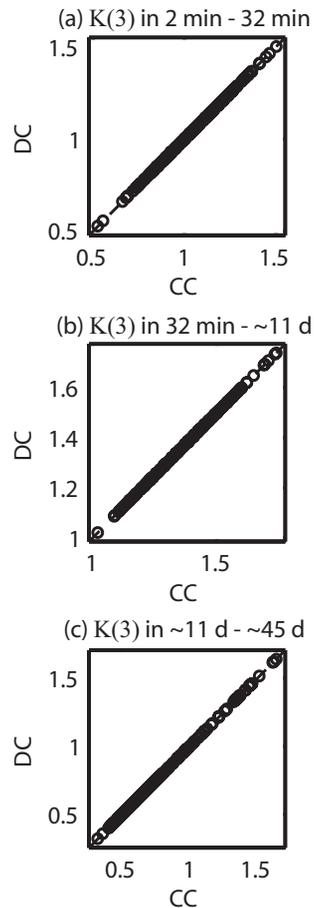
**Fig. 12.** Scatterplots between the multifractal exponents  $K(3)$  computed from the signal sampled with CC (x-axis) and DC (y-axis) methods. Each panel refers to a given scaling regime.
