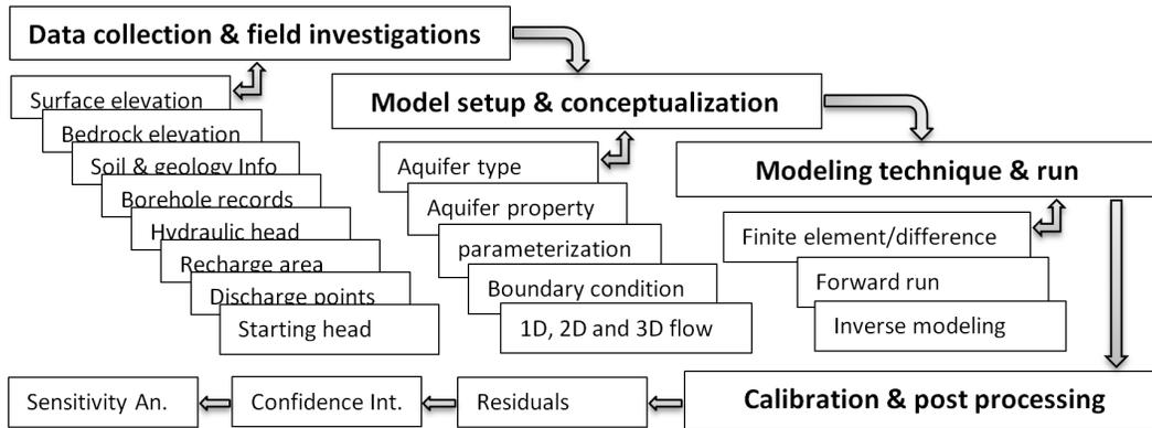
**Fig. 3.** Flow chart of a mathematical groundwater model.
