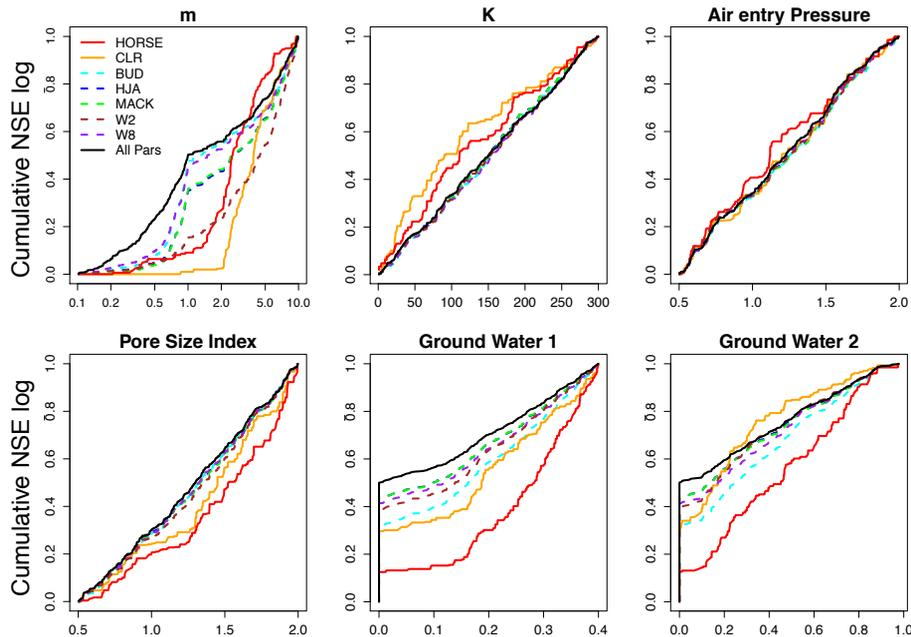
**Fig. 3.** Cumulative distribution of performance across parameter sets. Solid black line shows the original parameter distribution; colored lines show distribution of performance by parameter value for each watershed. Departures from the black line show preference for particular parameter values.
