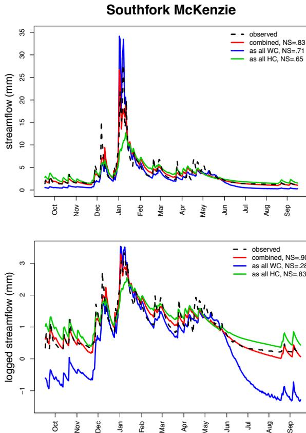
**Fig. 5.** Observed and modeled daily (a) streamflow and (b) log-transformed streamflow for Southfork McKenzie. Modeled streamflow estimates are shown for three parameter-transfer strategies including using only WC end-member parameters, only HC end-member parameters and combined strategy where parameters are varied spatially according to HC/WC geologic classification within the Southfork watershed.
