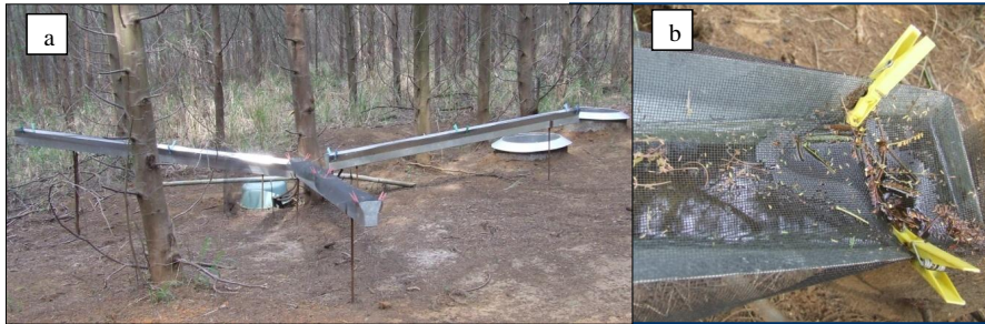
Fig. 3. (a) Throughfall troughs with mosquito netting covering; (b) showing the blockage of a trough.
