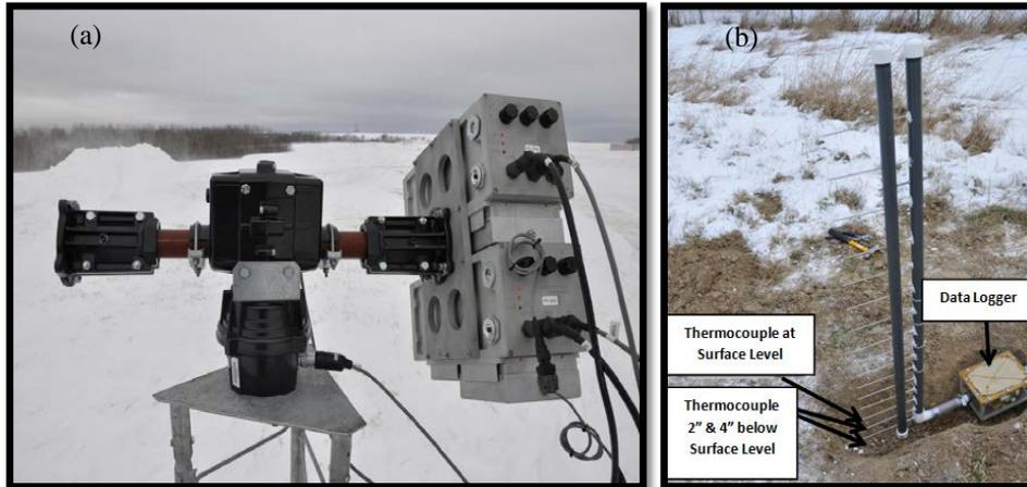
**Fig. 2.** (a) Microwave Radiometer (37 and 89 GHz) attached to automatic azimuth positioner. (b) Temperature profiler with 16 Watlow Rigid Sheath Thermocouples to measure air/snow temperature at defined depths.
