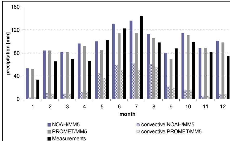
**Fig. 8.** Monthly convective and total precipitation of MM5 simulations coupled with NOAH and PROMET compared to measurements.
