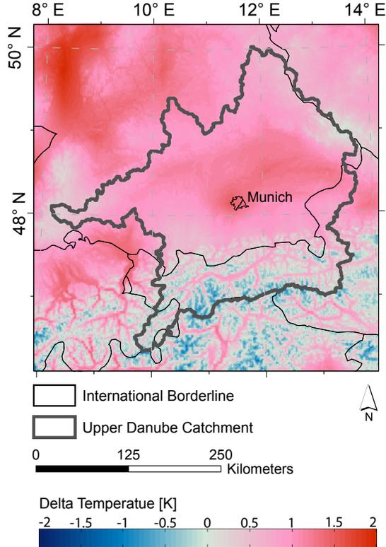
**Fig. 5.** Difference plot between PROMET/MM5 and NOAH/MM5 annual mean near surface air temperature in the Upper Danube Basin, downscaled to 1 km.
