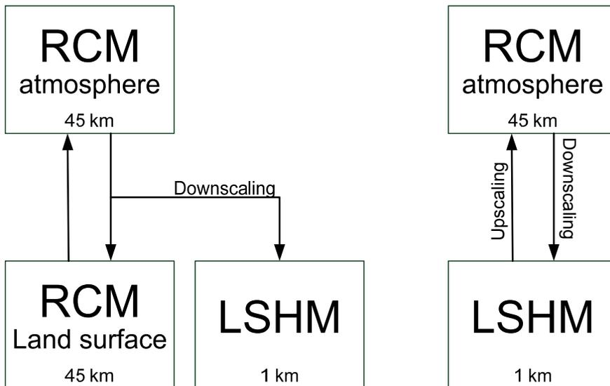
**Fig. 1.** Schematic illustration of 1-way (left) and 2-way coupling (right) a LSHM with a RCM.
