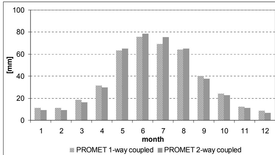
**Fig. 10.** Monthly mean evapotranspiration in the Upper Danube Basin of 1-way and 2-way coupled PROMET simulations (1996–1999).
