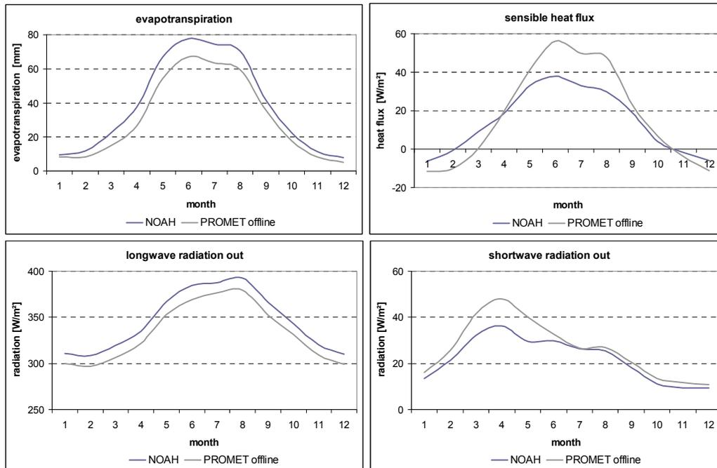
**Fig. 2.** Spatially averaged monthly land surface mass and energy fluxes (evapotranspiration, sensible heat flux, long-wave outgoing radiation, short-wave outgoing radiation) for the Upper-Danube catchment simulated with the NOAH-LSM and with PROMET offline respectively for the years 1996–1999.
