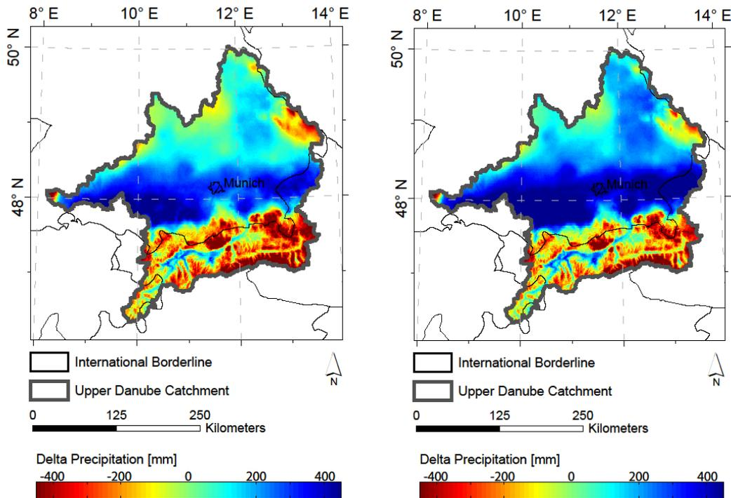
**Fig. 9.** Over- and underestimation of annual simulated PROMET/MM5 (left) and NOAH/MM5 (right) precipitation in the Upper Danube Basin, downscaled to 1 km and subtracted from measurements.
