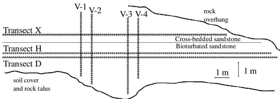
**Fig. 8.** Locations of nitrogen minipermeameter measurements along sandstone outcrop near Escalante, Utah. Modified after Castle et al. (2004).
