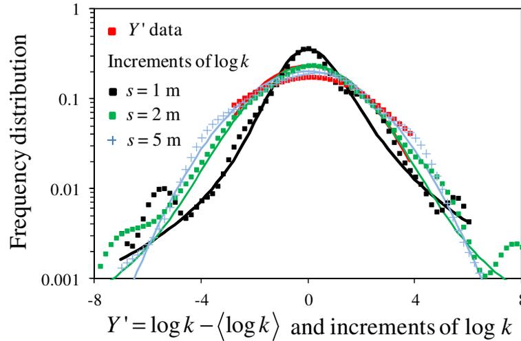
**Fig. 3.** Frequency distributions (symbols) and ML estimated probability density functions (curves) of (a) Arizona  $Y' = \log k - \langle \log k \rangle$  data (red) and  $\log k$  increments at lags  $s =$  (b) 1 m (black), (c) 2 m (green), and (d) 5 m (blue).
