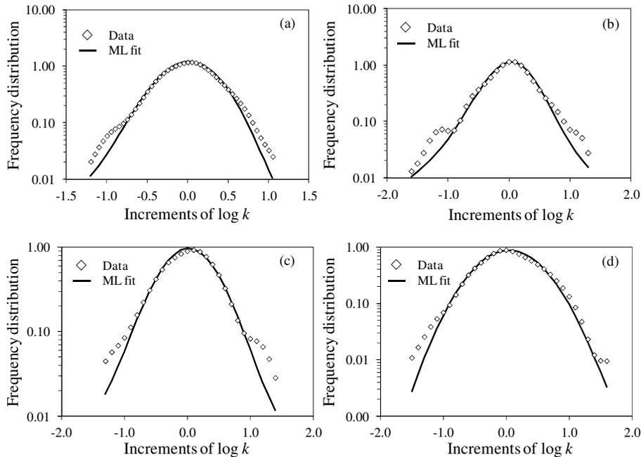
**Fig. 11.** Frequency distributions (symbols) and ML estimated probability density functions (curves) of Utah  $\log k$  increments along transects D and H at horizontal lags **(a)** 0.15 m, **(b)** 0.45 m, **(c)** 0.75 m, and **(d)** 1.5 m.
