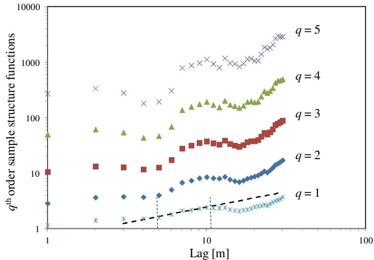
**Fig. 4.** Sample structure functions of orders  $q = 1, 2, 3, 4, 5$  of Arizona data versus lag. Light vertical broken lines demarcate midrange of lags within which heavy inclined broken line, with slope taken to represent  $\xi(1)$ , was fitted to  $S_N^1$ .
