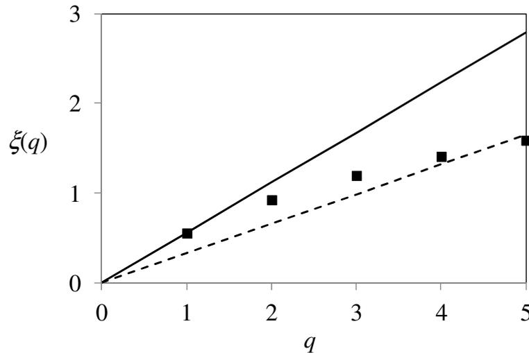
**Fig. 7.**  $\xi(q)$  as a function of  $q$  (symbols) obtained via ESS based on  $\xi(1) = 0.56$  computed for Arizona data by method of moments. Solid line has slope  $\xi(1) = 0.56$  and dashed line slope  $H = 0.33$  estimated for these data based on our theory, using maximum likelihood, by Riva et al. (2012).
