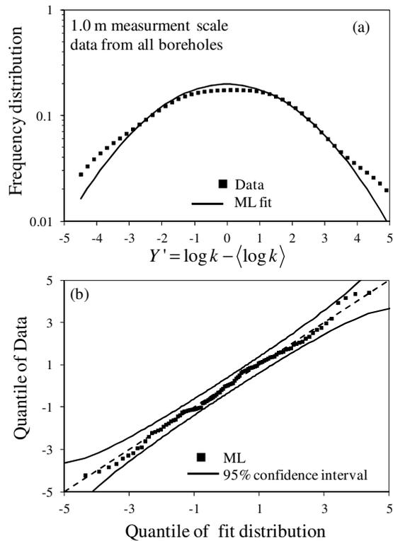
**Fig. 2.** (a) Frequency distribution (symbols) and ML estimated probability density function (solid curve) of Arizona data; (b) Q-Q plot of empirical data versus theoretical estimate of stable distribution.
