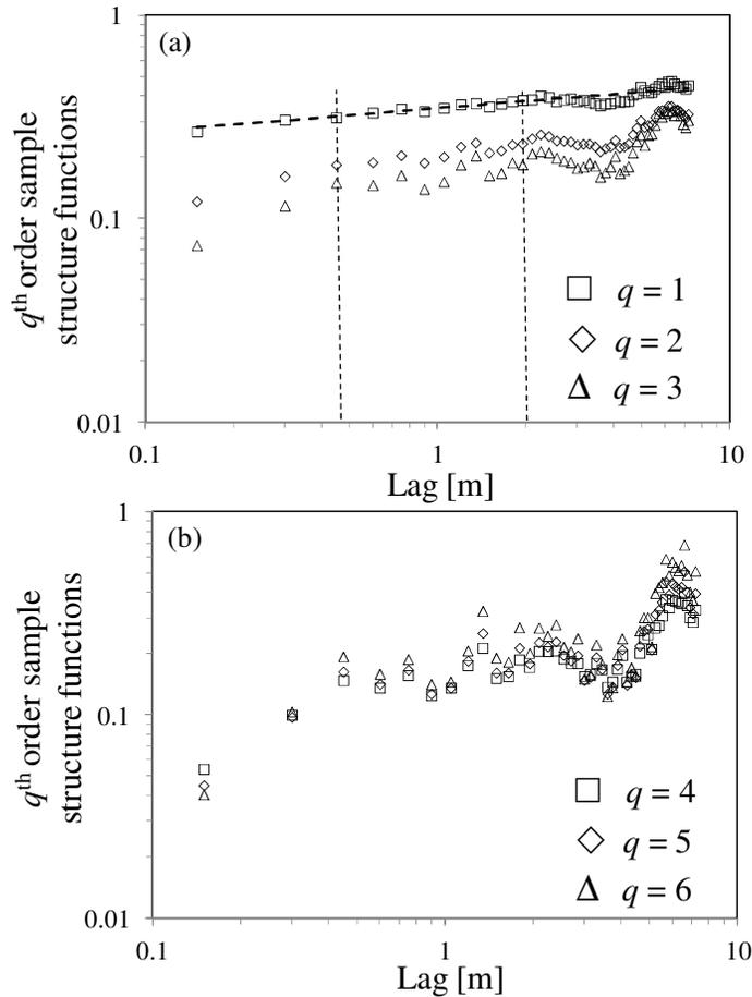
**Fig. 13.** Sample structure functions of order  $q = 1, 2, 3, 4, 5, 6$  of Utah data. Light vertical broken lines demarcate midrange of lags within which heavy inclined broken line, with slope taken to represent  $\xi(1)$ , was fitted to  $S_N^1$ .
