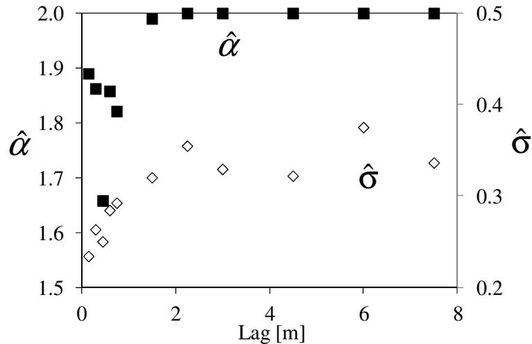
**Fig. 10.** Variations of ML Lévy index estimates  $\hat{\alpha}$  and scale parameter estimates  $\hat{\sigma}$  of Utah log permeability increments with horizontal lag along transects D and H.
