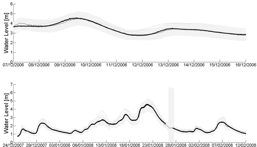
**Fig. 5.** Examples of 6 h ahead forecasts given at Welshbridge for two large flood events during calibration (upper pane) and validation (lower pane) periods generated using the DT model calibrated using the Gaussian methodology. The shaded area represents the 95 % prediction confidence interval with the solid line the expected value of the predictions. Observed data points are also shown.
