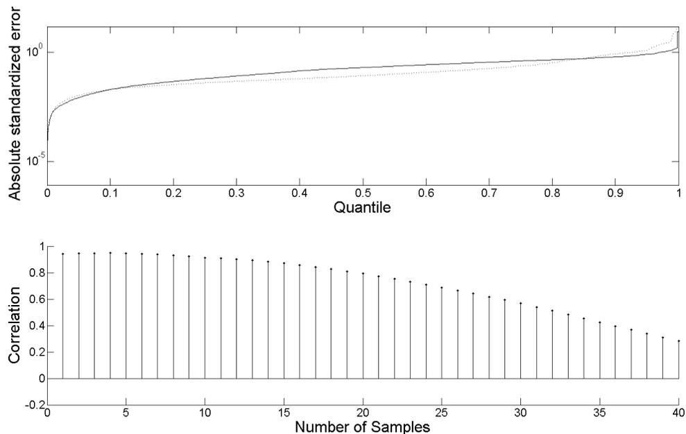
**Fig. 4.** Summary plots of the analysis of the 6 h forecast residuals for the RW model calibrated using the SEFE methodology. The upper pane shows the quantiles of the absolute values of the residuals. The solid line being positive residuals and the dotted line being negative residuals. The lower pane shows the auto-correlation of the residuals.
