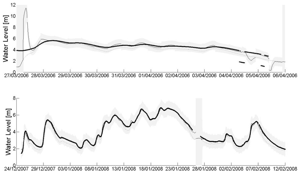
**Fig. 6.** Examples of 6 h ahead forecasts given at Llanrinio for two large flood events during calibration (upper pane) and validation (lower pane) periods generated using the RW model calibrated using the Gaussian methodology. The shaded area represents the 95 % prediction confidence interval with the solid line the expected value of the predictions. Observed data points are also shown.
