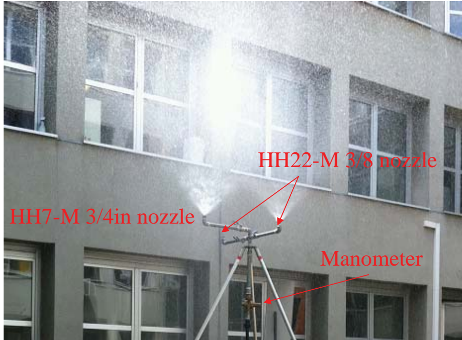
Fig. 4. View of the rainfall simulator. Water jets are sprayed from two HH22-M 3/8 in and one HH7-M 3/4 in nozzles.
