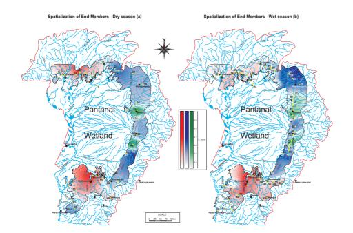
Fig. 8. Chemistry of river water at the border of the Pantanal wetland during DS 2008 (a) and WS 2010 (b), deducted from PCA-based EMMA procedure (green: end-member 1, blue: end-member 2, red: end-member 3; contributions above 35 % are drawn).
