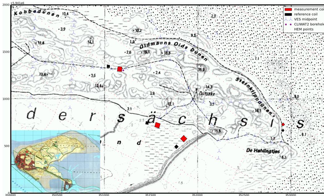
**Fig. 1.** Measuring area in the east of Borkum and location of MRS measurement (red) and reference (black) coils, VES midpoints (blue tri-stars), the CLIWAT 2 borehole (magenta) and HEM soundings (red dots) in the east dunes of Borkum.
