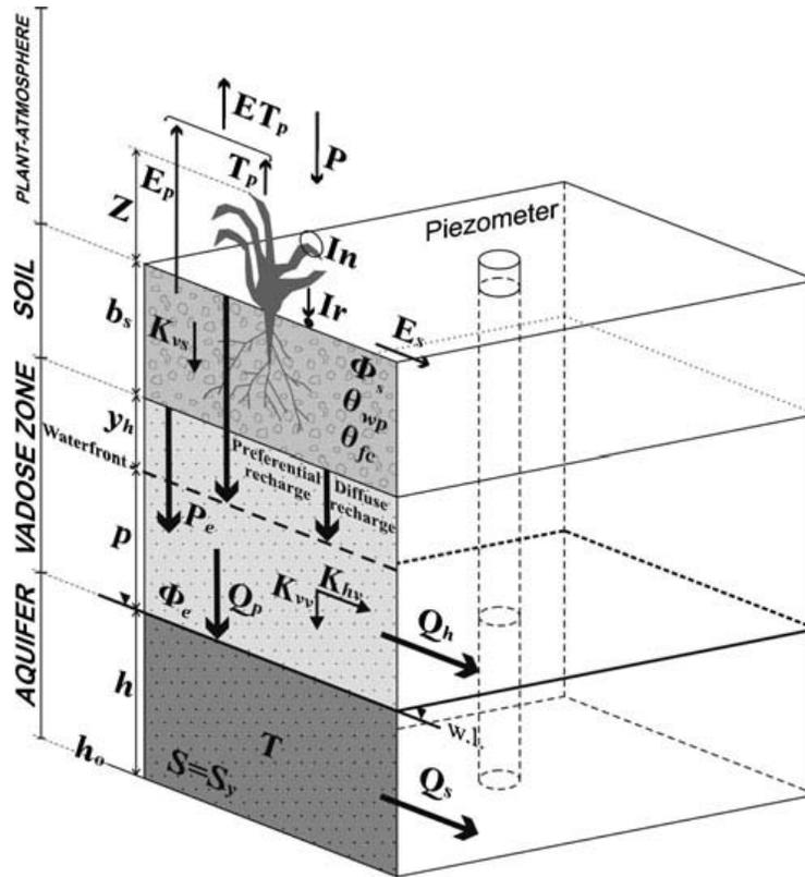
**Fig. 2.** Main components of water budget considered under the framework of the computer program Visual Balan (Samper et al., 2005; Jiménez-Martínez et al., 2010).
