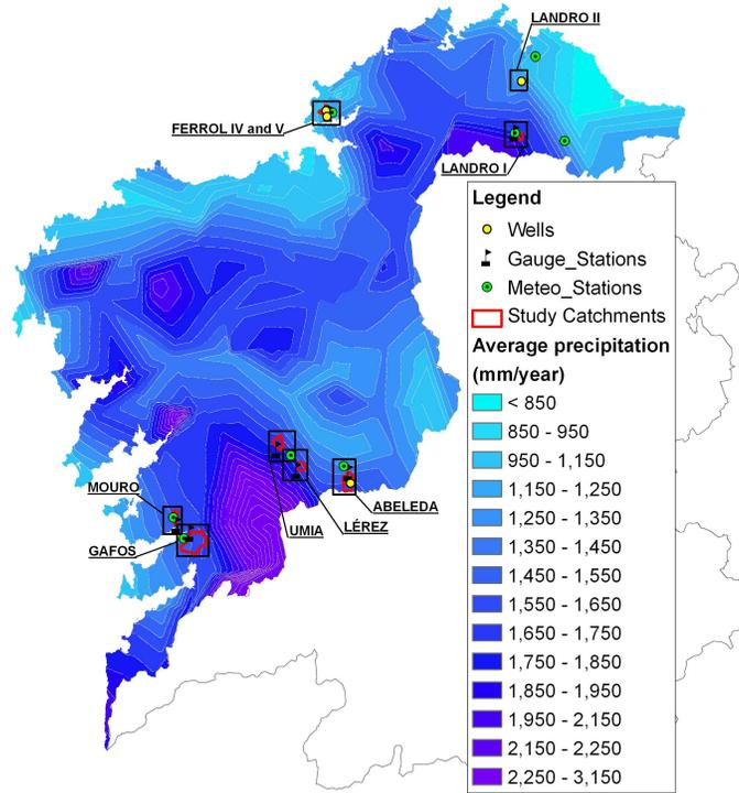
**Fig. 3.** Location of weather stations, wells and discharge gauge stations used for modeling the study catchments, and average precipitation map for Galicia-Costa built with data from Hydrological Plan of Galicia Costa (Xunta de Galicia, 2003).
