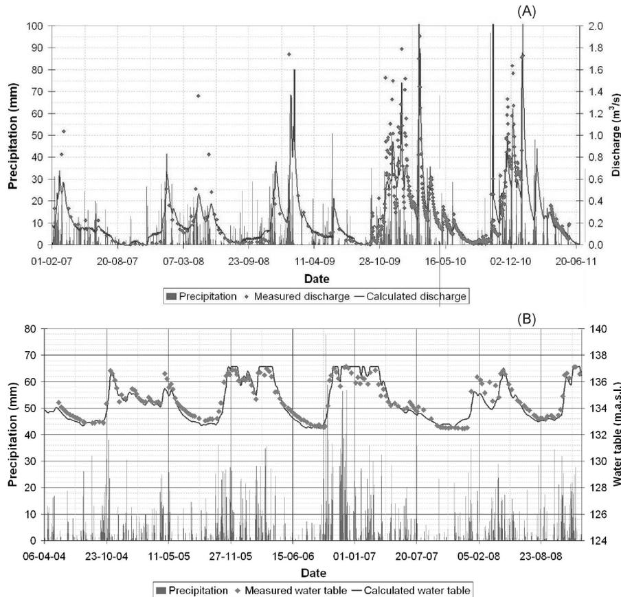
**Fig. 4.** Modeled versus measured flow rates in Abeleda Catchment **(A)** and modeled versus measured water table levels in Ferrol V Catchment **(B)**.
