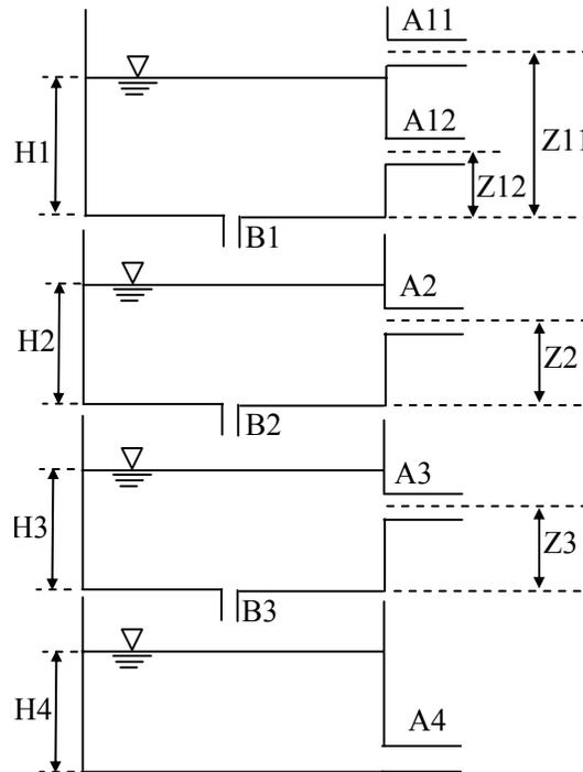
**Fig. 2.** Tank model structure for runoff estimations.
