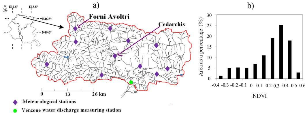
**Fig. 1.** (a) Catchment area representative of the Venzone water discharge measuring station and the distribution of meteorological stations within the study area. (b) NDVI composition of the catchment area derived from Landsat images taken on 29 July 2002.
