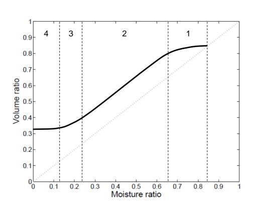
Fig. 1. Theoretical soil shrinkage characteristic curve, including 4 shrinkage phases.
