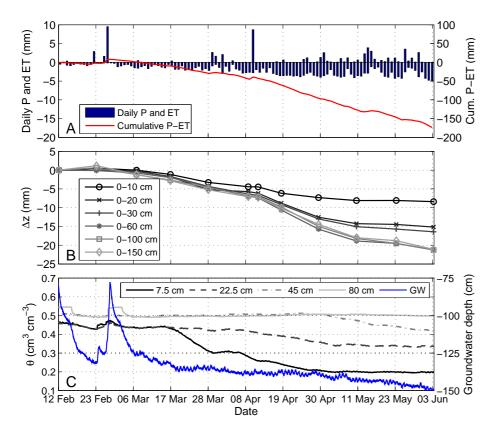
**Fig. 4.** Daily precipitation, daily evapotranspiration and cumulative net precipitation (**A**), cumulative layer thickness change  $\Delta z$  in six soil layers with respect to the starting date (**B**), volumetric soil moisture content  $\theta$  from CS616 sensors at four depths and groundwater depth (**C**) at field A from 12 February until 3 June 2011.
