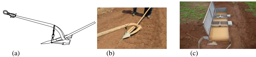
Fig. 3. (a) The traditional plow in Ethiopia, Maresha . (b) Winged subsoiler. The winged subsoiler has a vertical share and wings with sharp edges (MST, 2008). (c) Runoff trough used in the study. The picture was taken following a high rainfall day on 31 August 2010. About 2\text{ m}^3 (13 mm) of runoff was recorded by the trough from a 36\text{ mm d}^{-1} rainfall event on a field with TT wheat.
