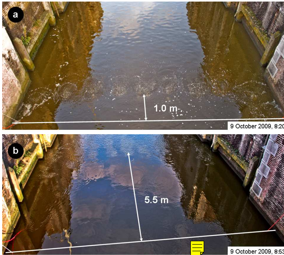
Fig. 8. The bubble envelope during low ( 3.3 \text{ m}^3 \text{ s}^{-1} ) and high ( 16 \text{ m}^3 \text{ s}^{-1} ) discharge, respectively.
