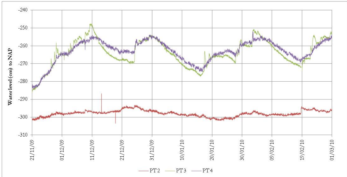
Figure 3 Measured groundwater levels in three of the piezometers (Pressure transducer 2 (PT 2) measures confined levels and PT 3 and PT 4 measure phreatic levels. PT 1 had to be discarded)
