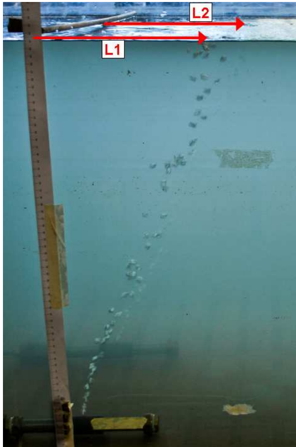
Fig. 5. Side view of the measurements in the laboratory flume; L1 represents the horizontal displacement of bubbles originating from the nozzle located near the flume's wall, L2 of the ones from the nozzle located in the middle.
