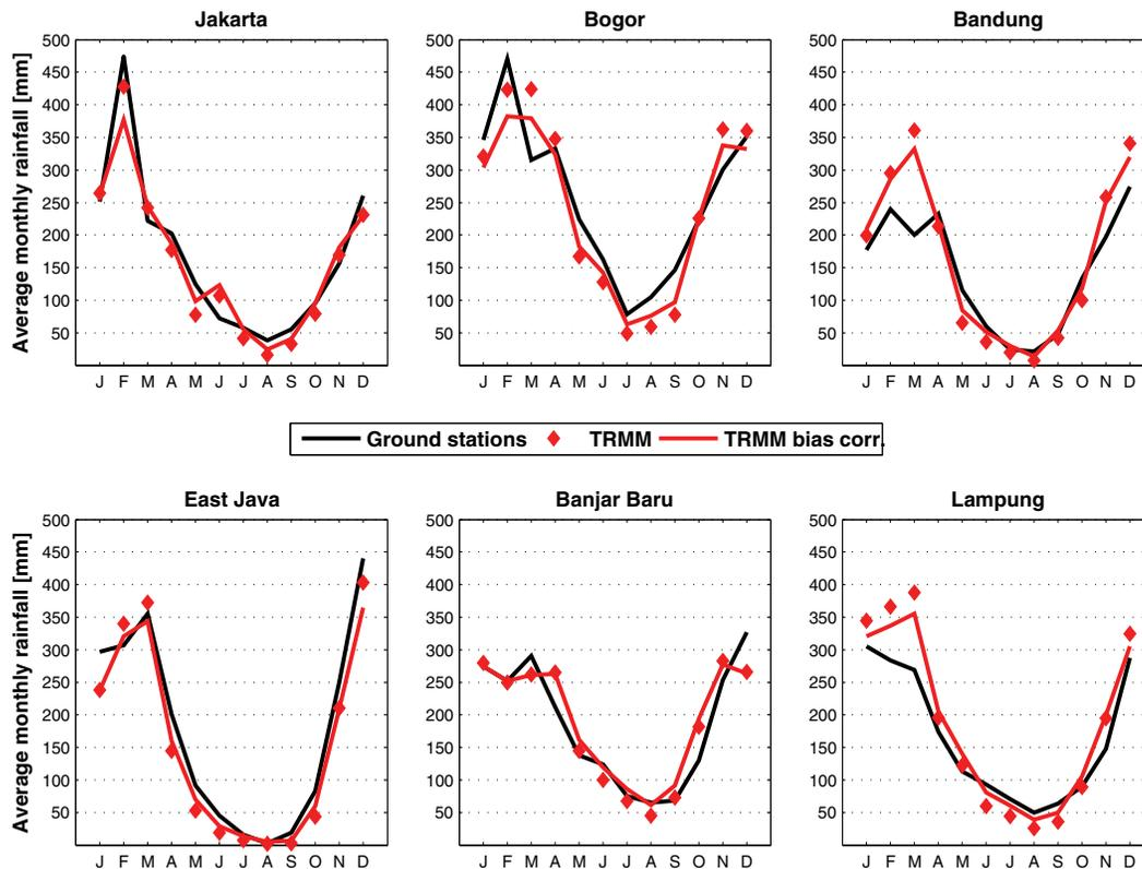
**Fig. 6.** Average monthly bias corrected TRMM data over 2003–2008, compared with ground station and uncorrected TRMM data.
