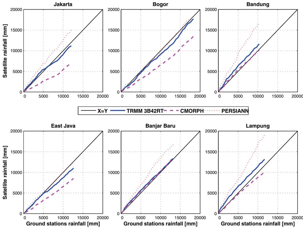
**Fig. 4.** Double mass curves showing the accumulated amount of rainfall of the observations against the satellite estimates (TRMM 3B42RT, CMORPH and PERSIANN) for each of the six validation areas for 2003–2008.
