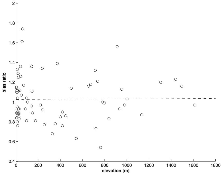
**Fig. 8.** Bias ratio vs. elevation for the individual ground stations in the six validation areas ( $R^2 = 0.0001$ ,  $n = 73$ ; of the 76 available stations (Table 1), 3 did not have any full year of validated observations).
