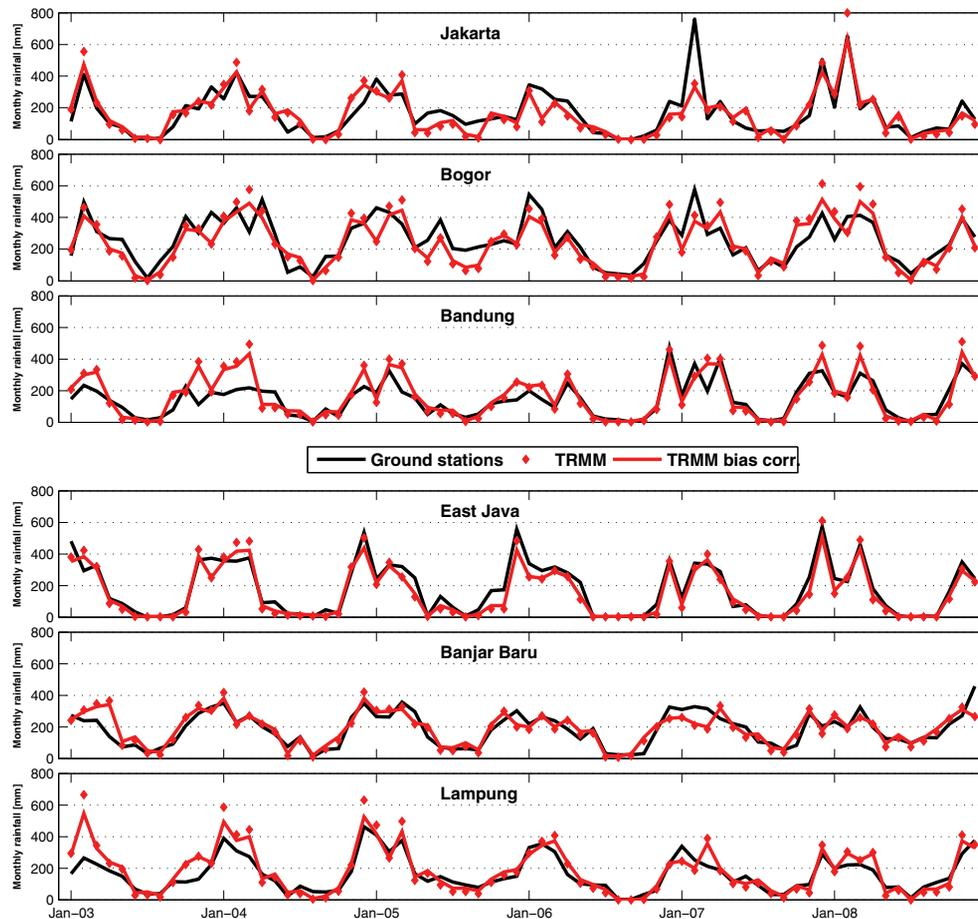
**Fig. 7.** Comparison of average monthly ground station rainfall with bias corrected and uncorrected TRMM 3B42RT for the individual validation areas.
