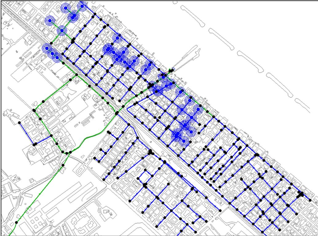
**Fig. 9.** Flooded network nodes resulting from the simulation of the most severe event occurred in year 2009 (event II in Table 1).
