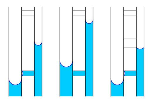
**Fig. 1.** Figure 1. Three tube systems consisting of cylindrical capillaries and throats. The middel throat in the RHS sketch has a radius between those of the vertical caillaries.
